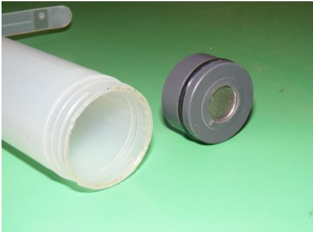
Figure 1. Initial CRD capsule and end-cap design
