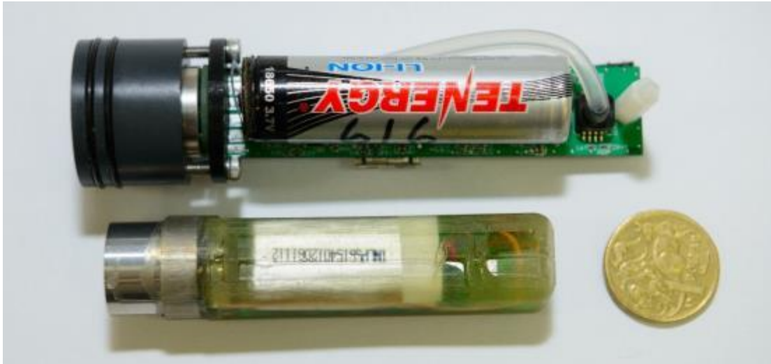
Figure 14. New PACP Pan wireless CH 4 and CO 2 IR gas-sensor device designed for sheep compared to the original PACP Serqet wireless CH 4 and CO 2 IR gas-sensor device
