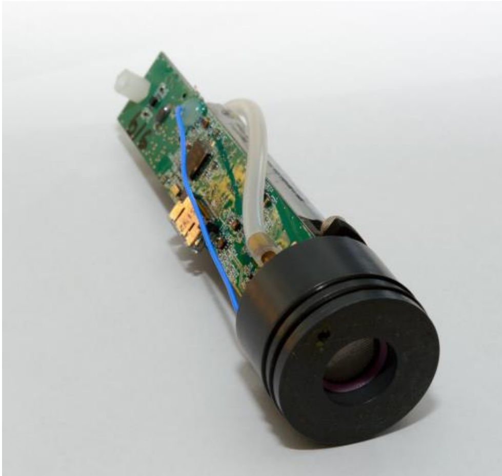
Figure 8. CH 4 and CO 2 IR gas-sensor device showing end-cap seals
