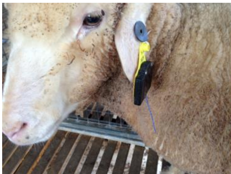
Figure 39. Configuration for Relay Experiment 5: Ear tag in the ear of a sheep with whip antennae extended and rumen node in the CRD with a whip antenna
