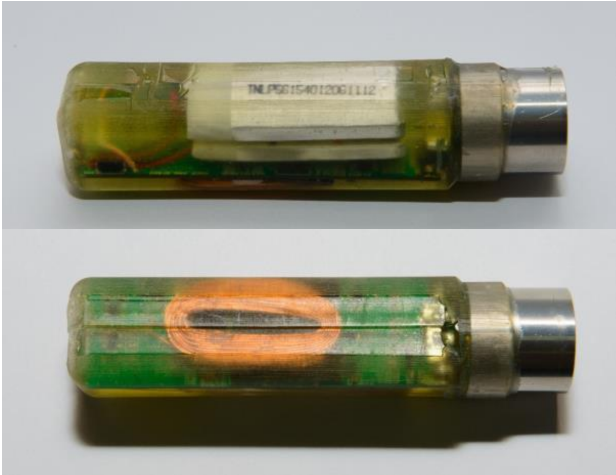
Figure 15. PACP Pan wireless CH 4 and CO 2 IR gas-sensor device showing batteries and the inductive charging coil
