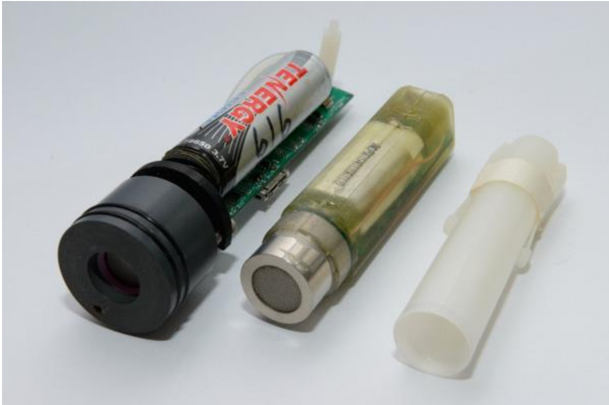
Figure 15. PACP wireless CH 4 and CO 2 IR gas-sensor devices and a sheep CRD
