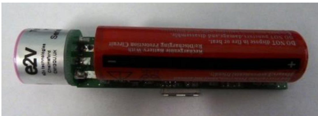
Figure 16. Original PACP Hydra wireless hydrogen intra-rumen gas sensor device
