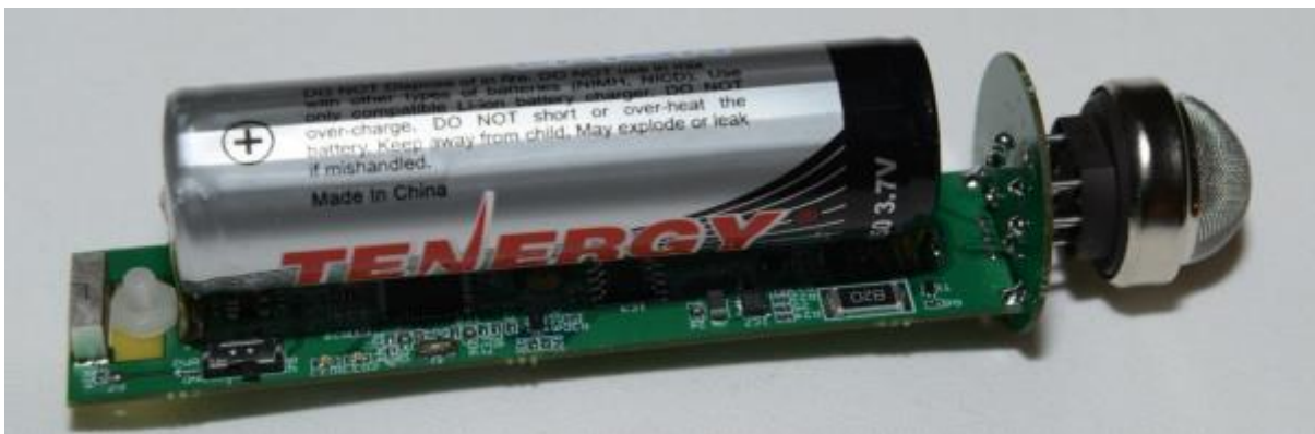
Figure 17. New PACP Hydra wireless hydrogen intra-rumen gas sensor device
