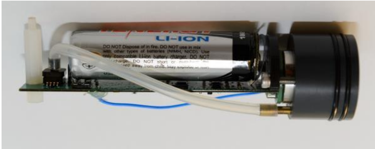
Figure 7. CH 4 and CO 2 IR gas-sensor device assembly
