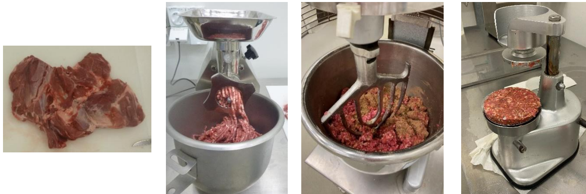
Figure 1: Process to manufacture lamb burger patties – lamb shoulder, mincing through 6 mm plate, mixing with spices, and forming the patties.
