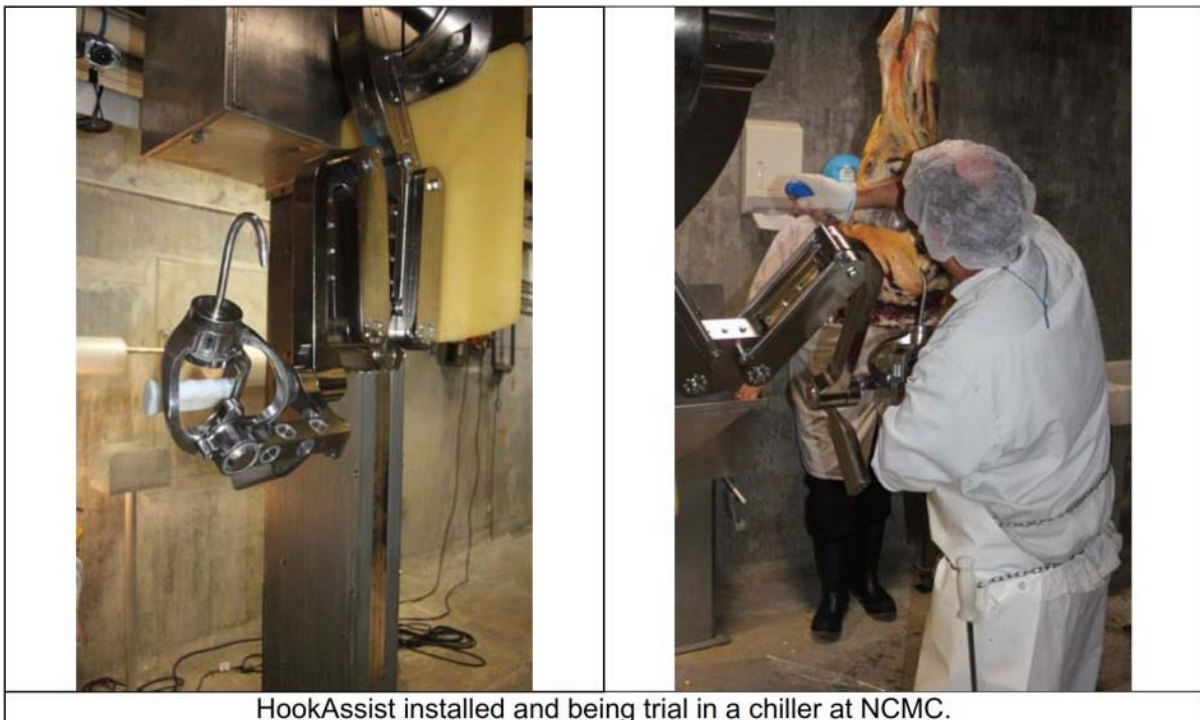
Figure 4: Hook Assist prototype system in industry trial sites
