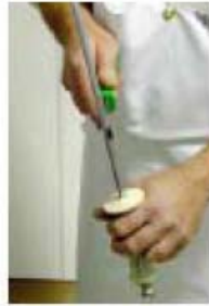
Check arm, steel and knife are square and in line. Knife handle centre of wrist
