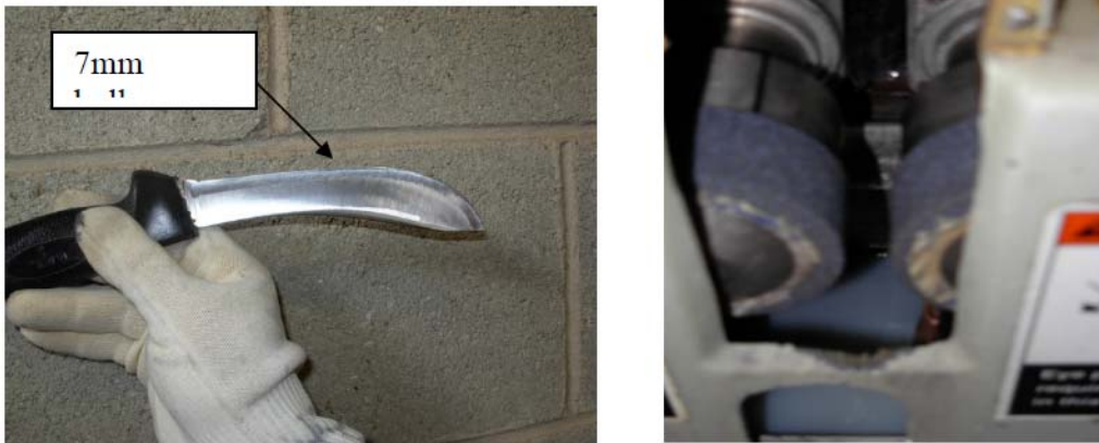
A perfectly hollow ground knife Pictures courtesy T&R Murray Bridge South Australia
