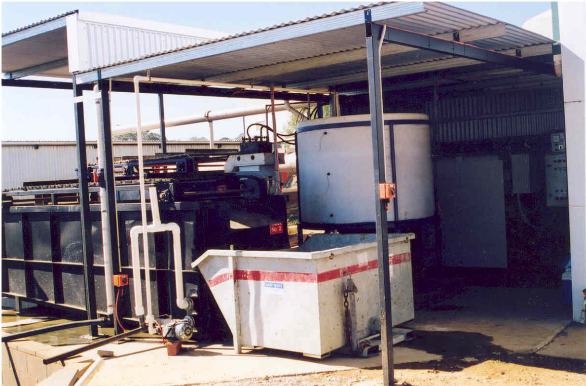
Figure 2: Electrocoagulation system at BMP, Young, NSW
