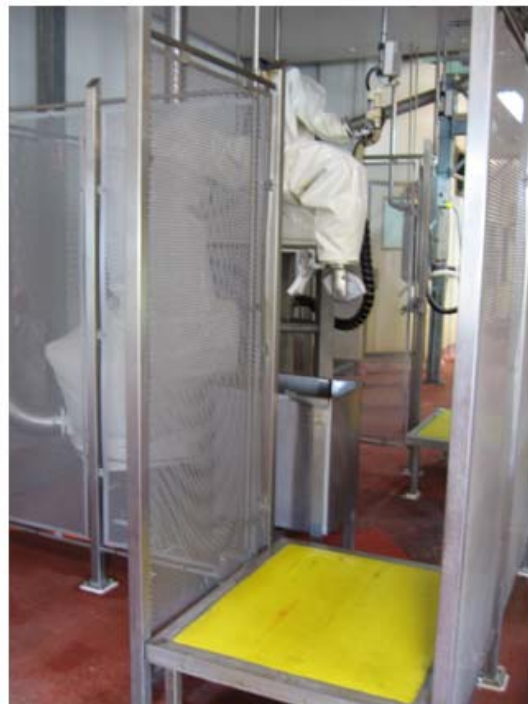
Fig. 4 Entry and exit safety mat platforms at GMP
