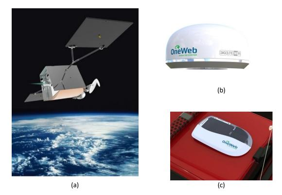
Figure 5-2. (a) Graphic of one of the proposed 648 LEO telecommunications satellites to be launched by U.S company OneWeb, (b) a user terminal for a building and (c) for a vehicle. Once linked to the LEO satellites, these act as a small cell, generating a 3G or LTE (and Wi-Fi) zone around it for an existing mobile network operator (Source: <u>http://oneweb.world/#technology</u>) (Extracted from Lamb, 2017).
