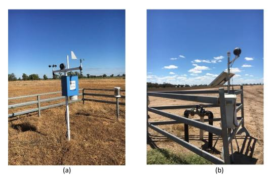
*Figure 3-11.* Two examples of automatic weather stations (AWS) located in feedlots incorporating mobile phone network links.
