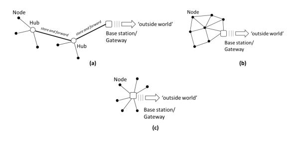
Figure 2-3. A basic network diagram as relates to (a) 'store and forward', (b) 'mesh', and (c) star farm sensor networks (Extracted from Lamb, 2017).
