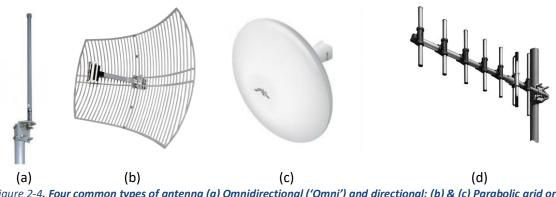
Figure 2-4. Four common types of antenna (a) Omnidirectional ('Omni') and directional; (b) & (c) Parabolic grid or dish (or semi-parabolic grid/dish) in two common forms and (d) Yagi (Source: (a) http://maxcomm.co.za; (b) http://www.l-com.com; (c) <u>www.ubiquiti.com</u> and (d) https://www.scmsinc.com).
