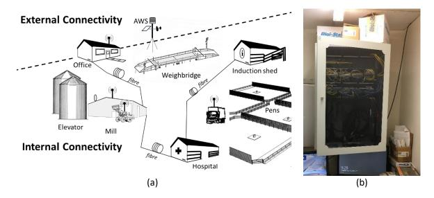
Figure 2-1. (a) An example schematic of a fibre loop installed in an Australian feedlot and (b) inside the feedlot office sits a network service cabinet; the heart of an internal fibre loop within the feedlot precinct.
