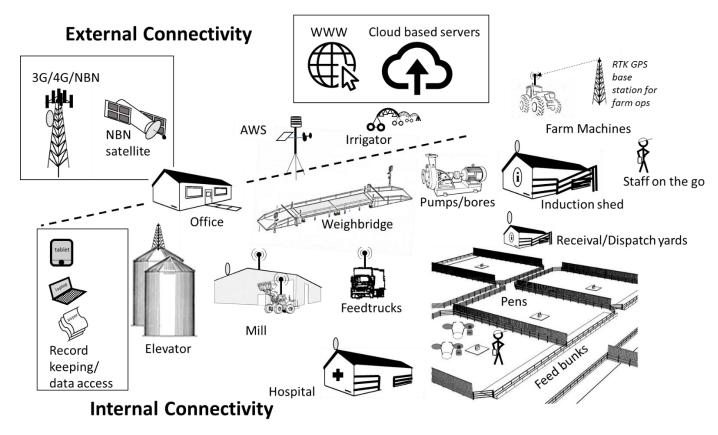
Figure 1-1. Some of the many data/information sources and consumers in a feedlot environment
