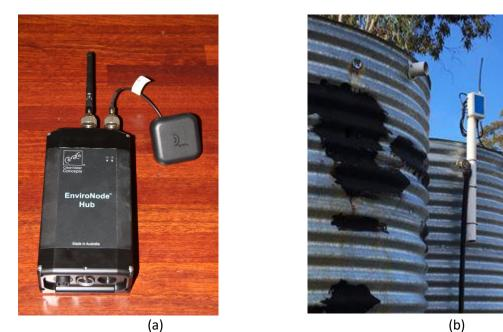
Figure 3-16. (a) An example of an Iridium IoT hub and (b) a Myriota-developed LEO satellite transmitter connected to a tank water level sensor. (Source: Ric Otton, Dosec Design and Tom Rayner, Myriota; extracted from Lamb, 2017).
