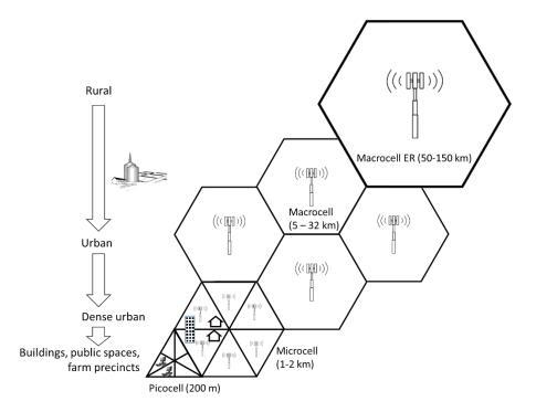
*Figure 3-5.* Basic mobile cell types. Indicative cell radius (in km) included (Adapted from MobileNetworkGuide 2016) (Extracted from Lamb, 2017)..
