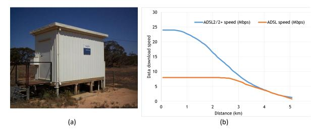
Figure 3-3. (a) A typical local exchange a seen in rural Australia (Source: Longhair, CC BY 2.5, <a href="https://commons.wikimedia.org/w/index.php?curid=3934601">https://commons.wikimedia.org/w/index.php?curid=3934601</a>) (b) ADSL and ADSL2+ download speeds relative to distance between subscriber and local exchange (Source: <a href="http://www.adsl2exchanges.com.au/">http://www.adsl2exchanges.com.au/</a>).
