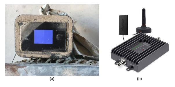
Figure 3-9. (a) Example of a small (shoe-box) sized cell booster used to create a zone of amplified signal strength in an around a building, in this case around a mill shed. The 'donor' antenna is located on the shed roof. (b) An example of a vehicle cell booster (www.ubersignal.com). Whilst cell boosters can increase the signal strength and hence provide improved call quality, they do not necessarily increase data speeds.
