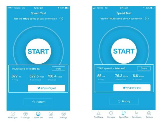
Figure 3-10. In the vicinity of two different feedlots, both within 15 km of nearby mobile network towers. Same handset, two different towers (including 3G and 4G), two different times, two different signal strengths and two entirely different outcomes in terms of speed. There are a multitude of factors that influence the relationship between signal strength and resulting (data) speeds.
