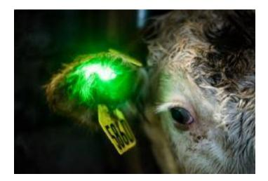
Figure 6-1. An example of a self-illuminating smart tag designed to provide pen riders a visual indicator of animal health (Source: Stewart McConarchy).
