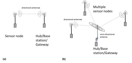
Figure 2-5. A basic wireless sensor network (WSN) indicating use of different antenna types used in (a) point-to-point and (b) point-to-multipoint links (Extracted from Lamb, 2017).
