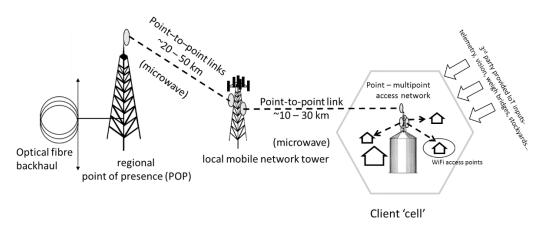
Figure 3-2. An alternative view of networks, especially relevant to some feedlots (discussed later) (Extracted from Lamb, 2017).
