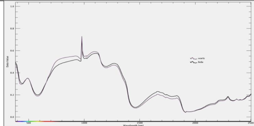
The spectra of the warts is almost identical to the spectra of the hide. Isolating these defects robustly will therefore be difficult using the spectral information from the hyperspectral camera. Augmenting with other vision processing algorithms may enable robust detection but this would need to be verified across a range of hide samples.
