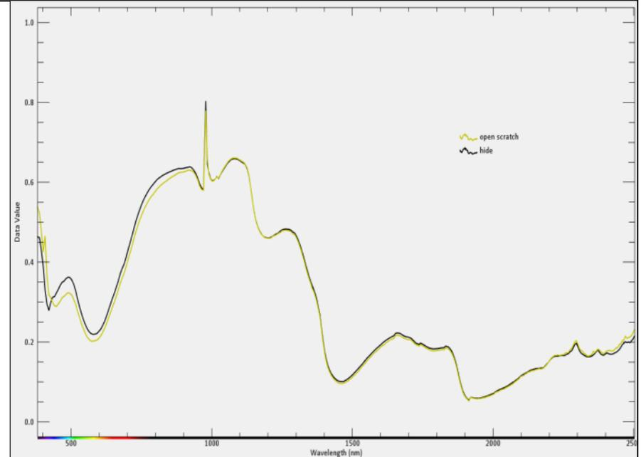
This will likely be confused for normal hide. The most likely reason for this is the spatial resolution was too low and a combination with motion blur washed out the physical defect. The spectra indicated no unique absorption bands on the pixels that appear to be the scratch.
