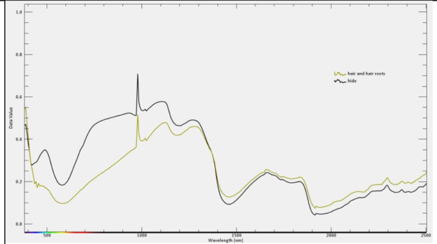
The spectra of the hair appear to be relatively unique from 700nm to 1300nm. It should be detectable and classified correctly depending on how homogeneous the hair spectra is.
