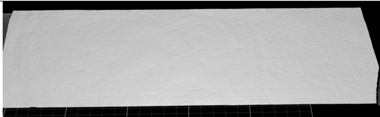
This is an image of the grayscale intensity of each pixel overlaid on the 3D surface of the hide.
