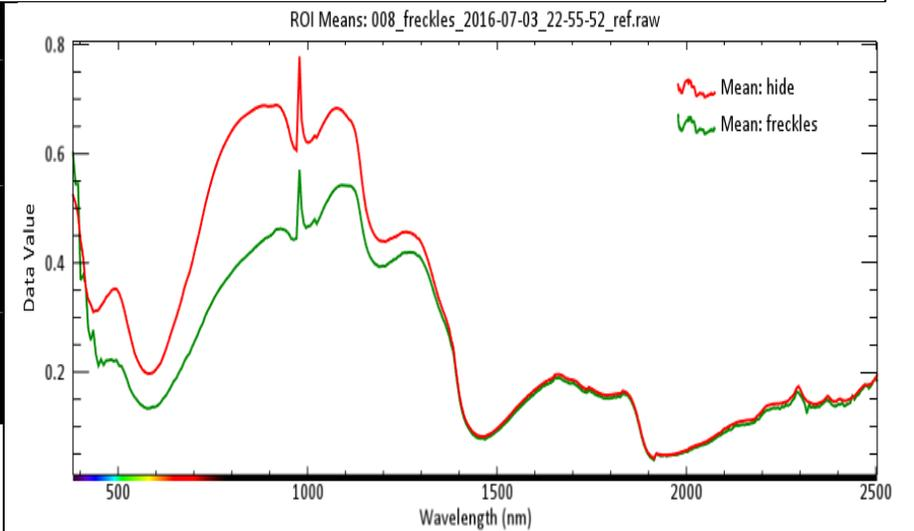
Freckles are likely to be confused for physical damage to the hide due to the fact that freckles possess some unique spectral properties. These will need to be taken into consideration to prevent false positive defect detection.
