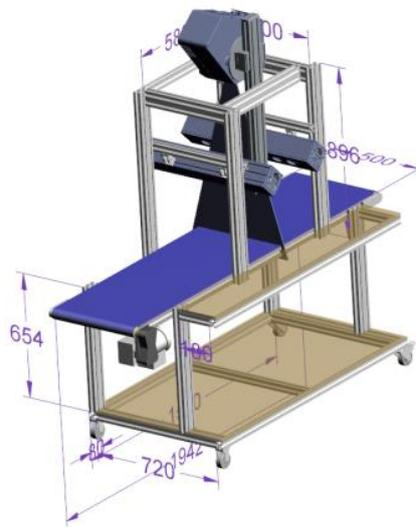
Figure 1 - Hyperspectral camera setup
