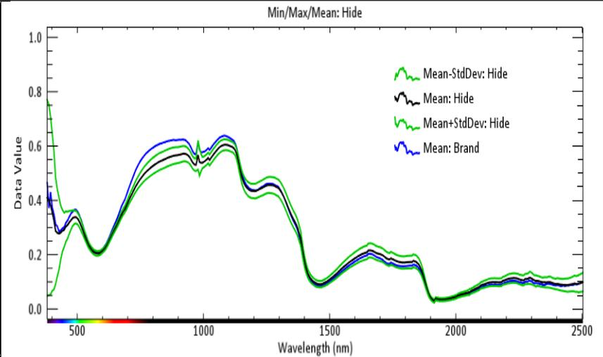
Spectra for the branding and spectra of clean hide. Note the first standard deviation illustrated by the green lines.
