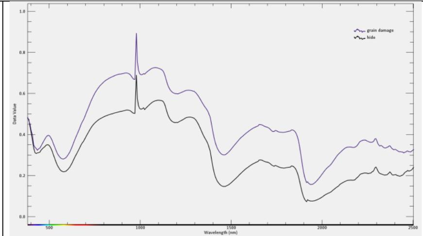
There are no characteristics of this spectra that strongly and uniquely define this defect from clean hide. Vision processing algorithms, in conjunction with spectral analysis algorithms, may be able to provide a result with this defect. Care will have to be taken however that these algorithms were robust enough to not introduce false detection in clean hide.
