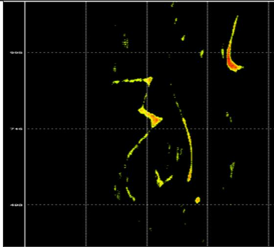
This is the best processed result of the hide. The image was generated by calculating the gradient from 580nm to 764nm then thresholding the image.
