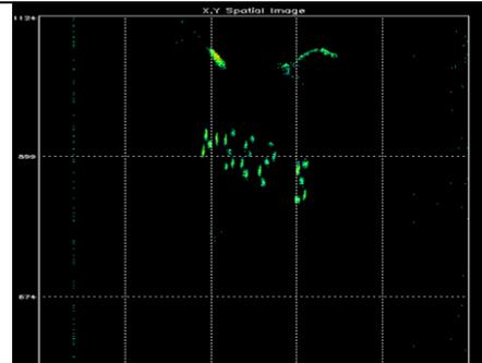
This is a processed result of the hide. The image was generated by calculating the gradient from 820nm to 950nm then thresholding the image.
