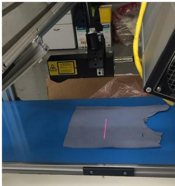
Figure 2 - 3D camera setup for hide profiling
