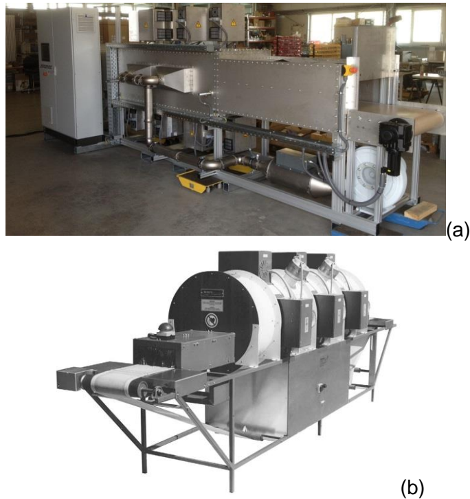
Figure 30. Microwave conveyor belts (a) Frickle and Mallah continuous microwave heating systems, (b) 4.5m continuous microwave belt furnace (Source: Vega-Mercado et al., 2001).
