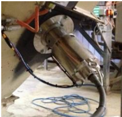
Figure 25. In-line NIRS of sorghum during processing measuring ground sorghum moisture concentrations. The measured values are blue lines with limits of orange warning lines and red alarm lines. The photo is of an installed Bruker in-line NIR emission head (Source: Courtesy of I Ward, Agri-Torque, 2016).
