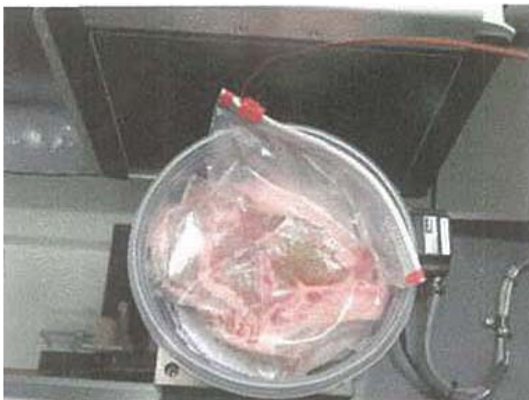
Figure 4. Meat sample on rotation stage in front of detector.
