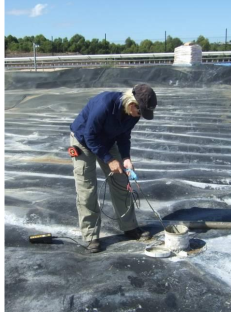
Photo 6: Crust measured with Royce Probe
