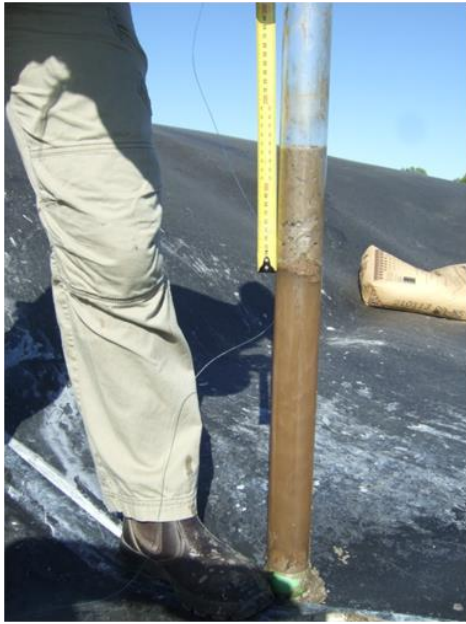
Photo 5: Crust measured with Perspex tube
