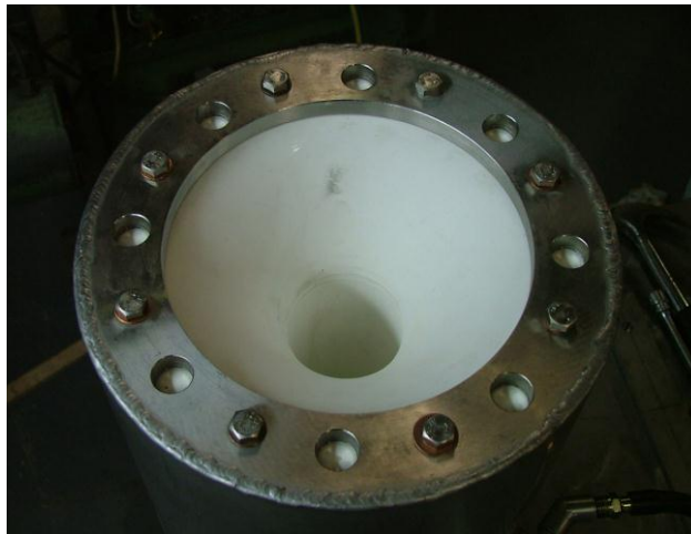
Figure 2. Commercial prototype meat stretching and shaping device. Top view of insertion of end of the cylinder – vacuum off.
