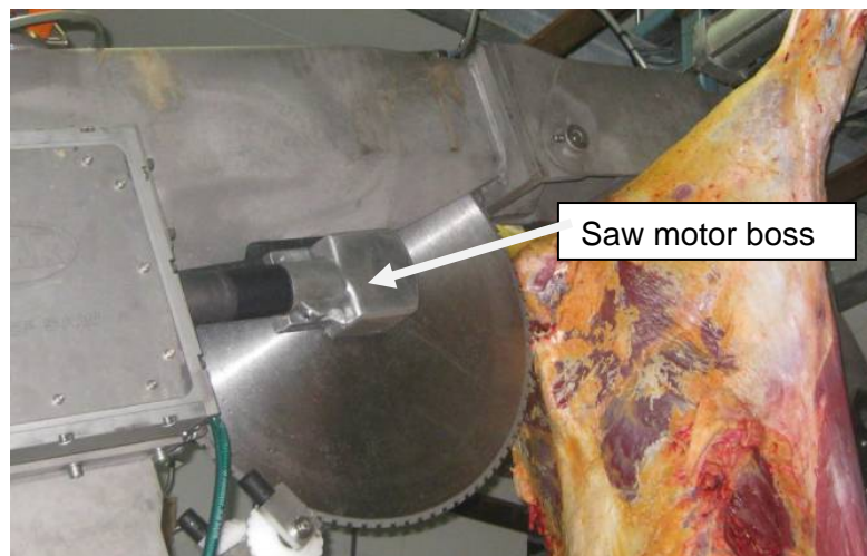
Fig 9 Saw motor Boss on one side of the saw blade
