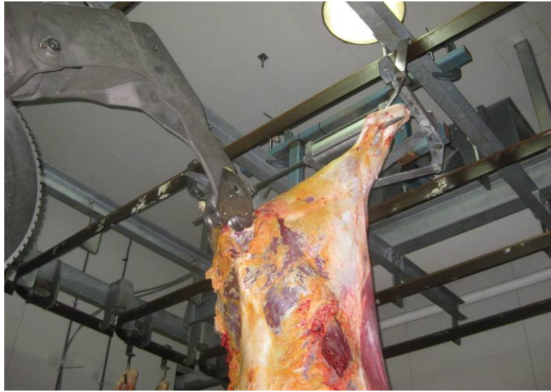
Fig. 8 Carcase Leg Spreader setup at ECT
