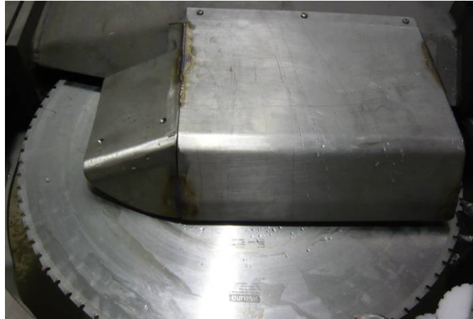
Fig.12 Guarding to eliminate carcass skew
