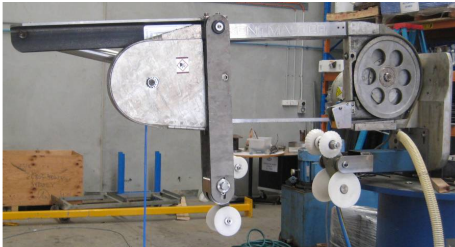
Fig.15 Bandsaw with Guidance Mechanism fitted
