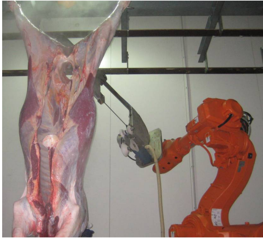
Fig. 16 Setup with Bandsaw at EC Throsby
