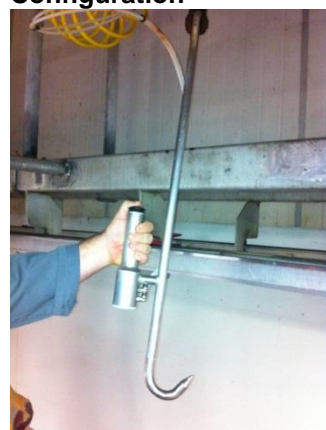
Figure 4: Pneumatic Assist for Higher Production Hook Swap
