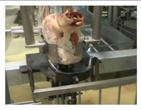
Step 2 – Integration robot transfers the middle section to the middle system loading fixture on the middle system carousel
