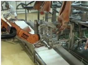
Step 1 – Primal system (Tower 1) removes forequarter from carcase
