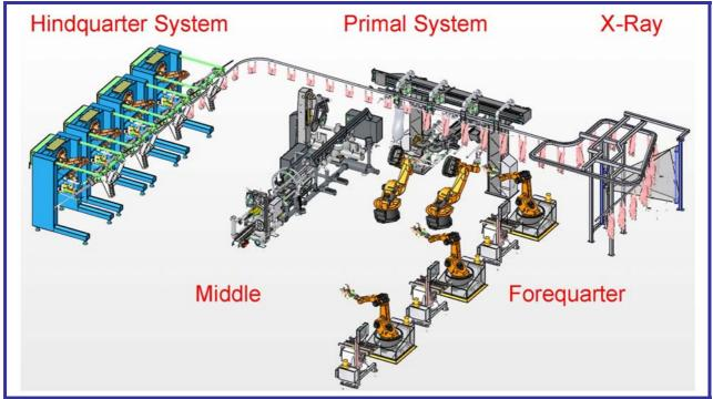
Figure 1: RTL Fully Automated Bone-In lamb Boning Solution
