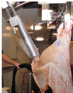
Fig. 3 Semi automated bagging of the bung
