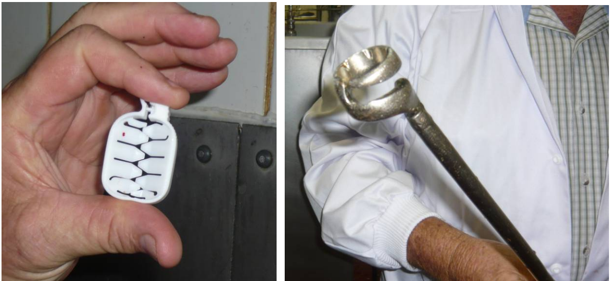
Fig.1 Rodding tool and Weasand Clip
