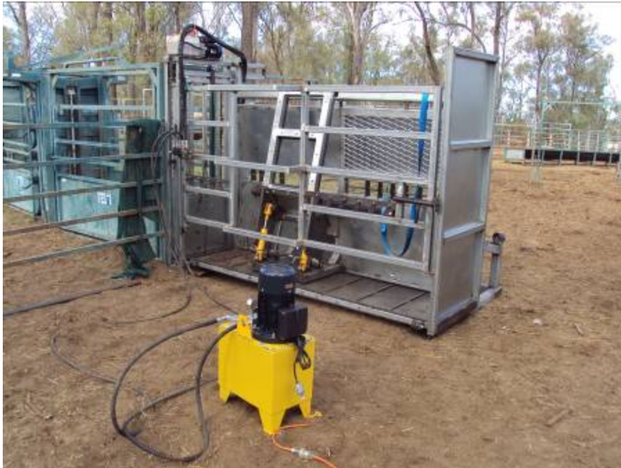
Figure 2 – Testing hydraulic Mark 4 restraining box at Start Engineering
