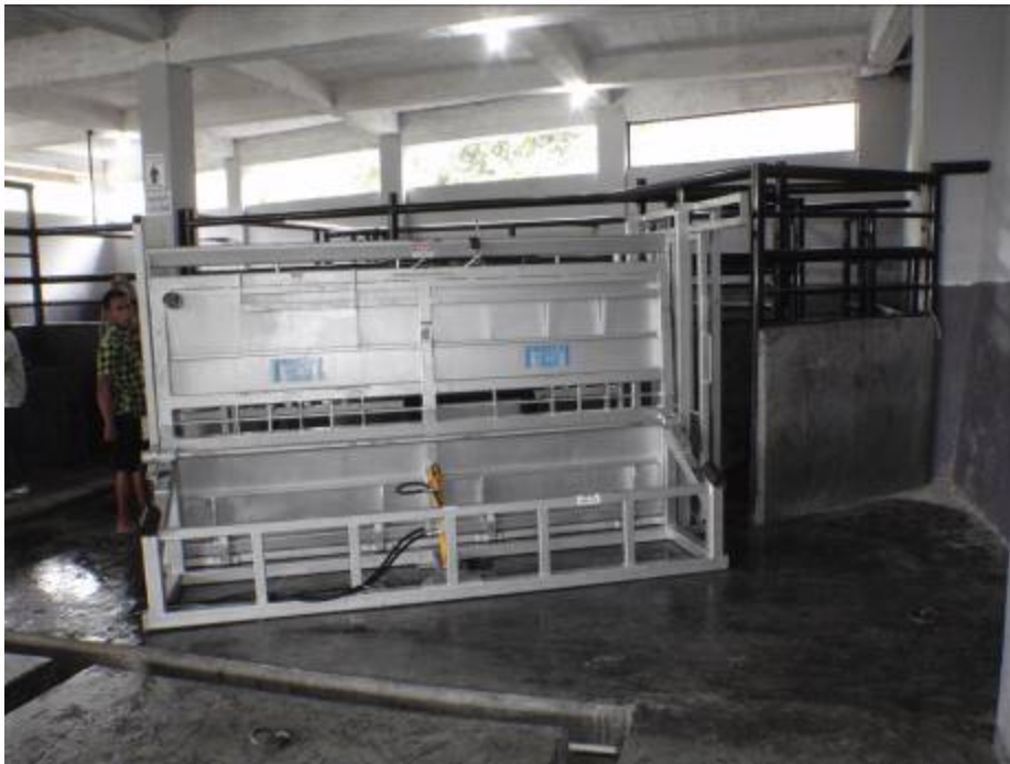
Figure 5 – Installing prototype manual Mark 4 restraining box (Lampung, Indonesia)
