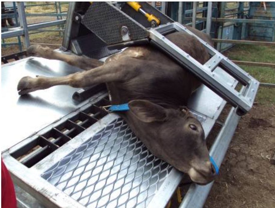
Figure 3 – Testing hydraulic Mark 4 restraining box at Stark Engineering
