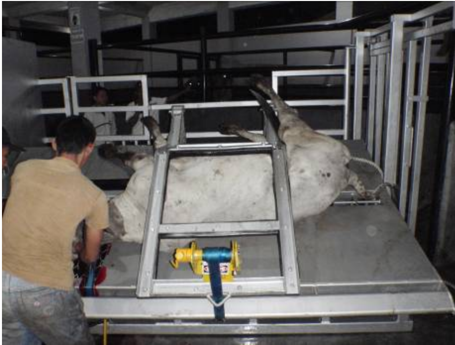
Figure 6 – Testing manual restraining box in Indonesian abattoir (Lampung)
