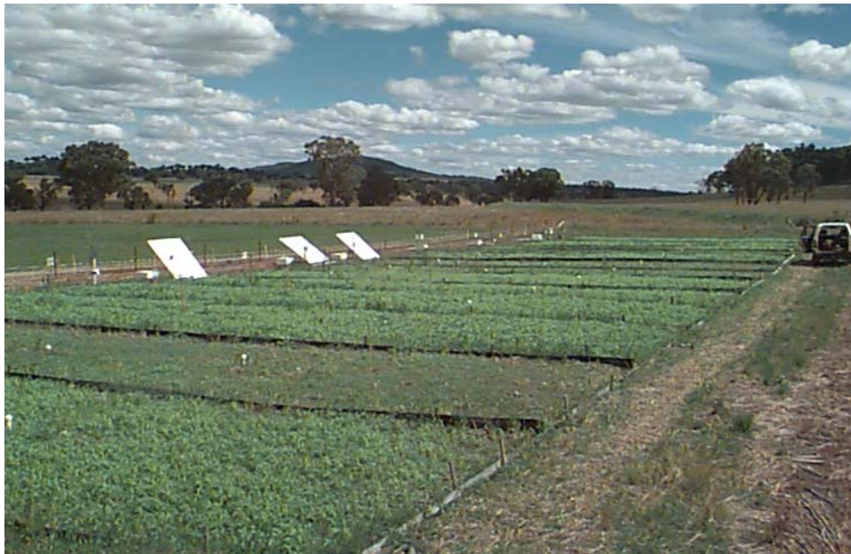
Figure 7: Experimental site showing plots, and raised lids of the instrumentation pits where tipping buckets are located. White boxes located next to instrumentation pits contain data loggers and counters.
