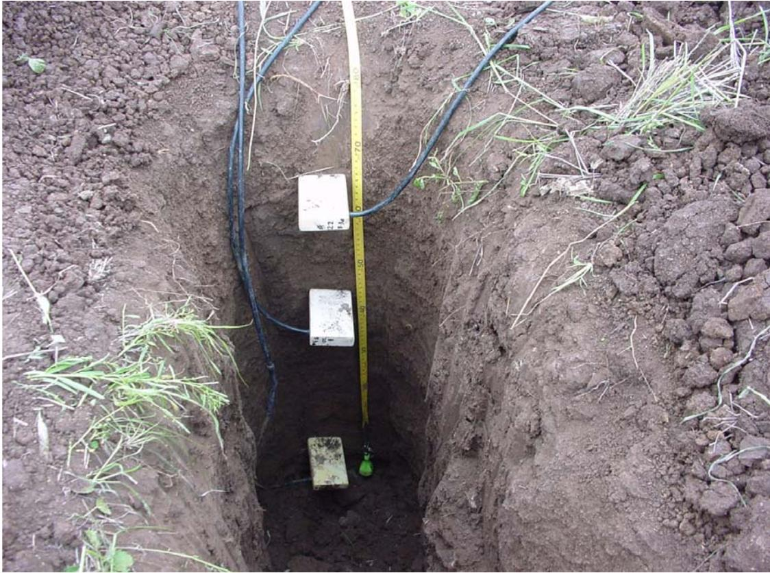
**Plate 4.4.2.** Installed soil moisture sensors at depths 15cm, 40cm and 80cm.
