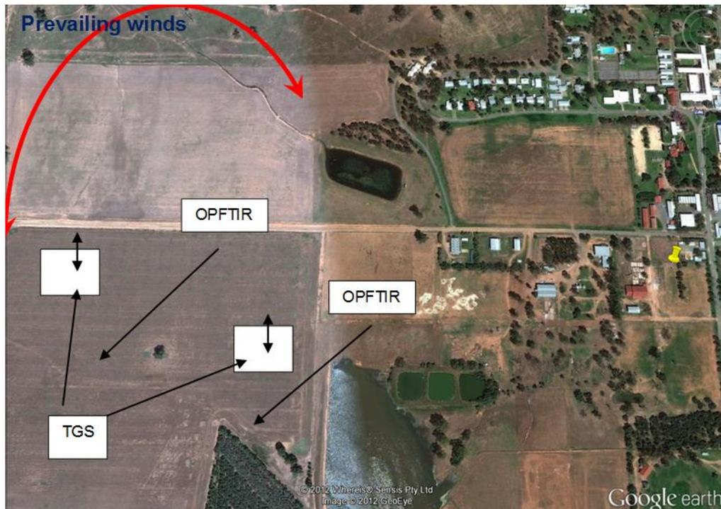
**Figure 3 Generalised plan of emissions measurements from feed lots**
