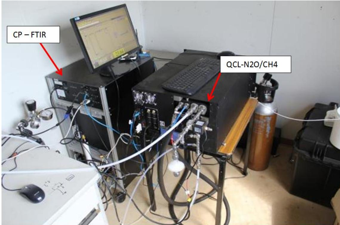
Figure 9 Close path N2O and CH4 analysers
