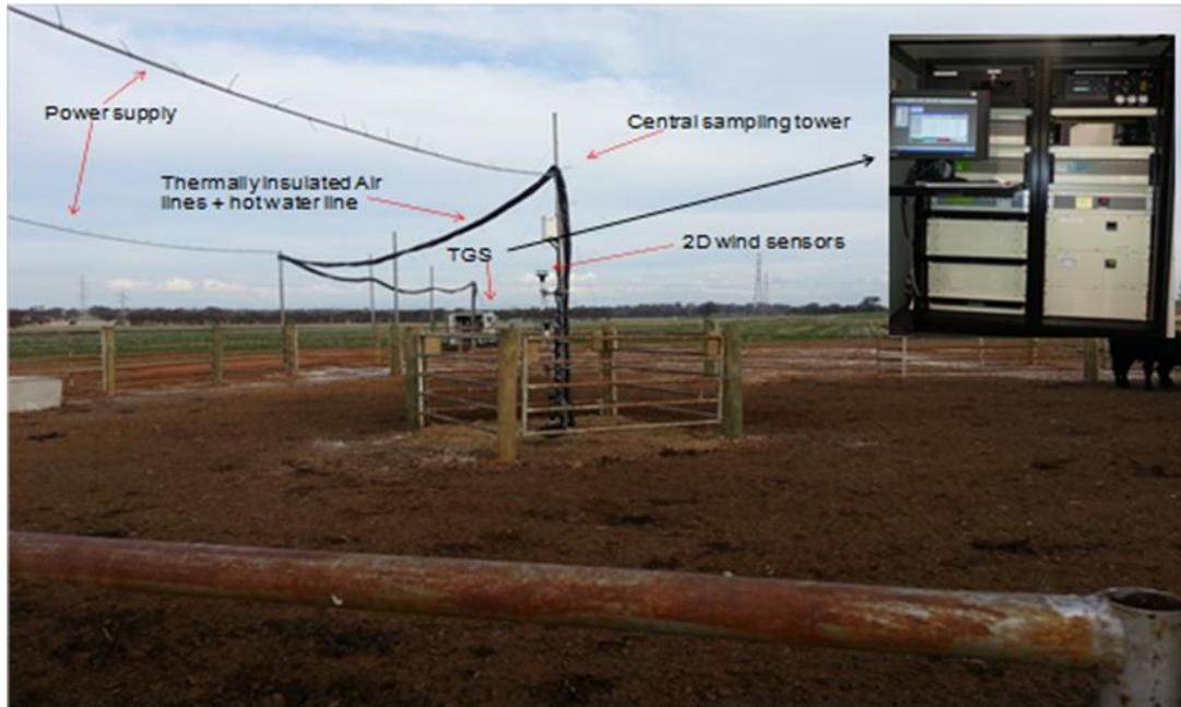
**Figure 4 Central gas sampling tower and air lines that delivered air samples to the trace gas analysis system**
