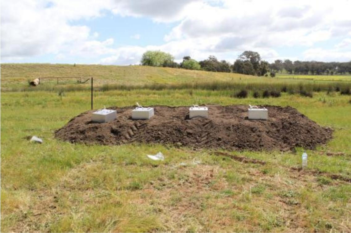
**Figure 6 Flux chamber measurements on manure piles**
