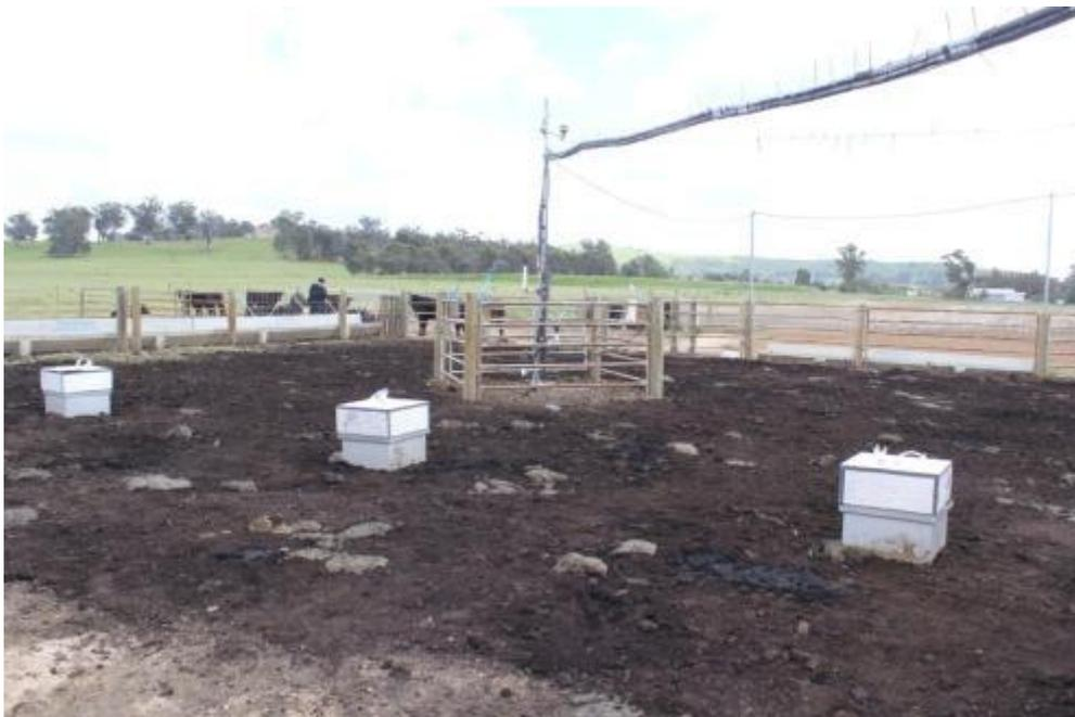
Figure 11 Flux chamber sampling at pen surface
