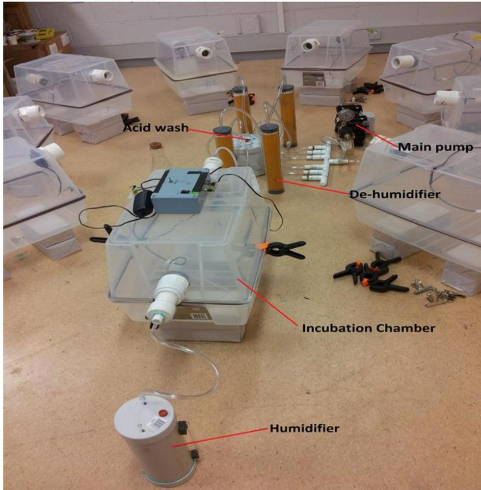
**Figure 1 Construction of new incubation chambers allowing 9 treatments to be run in parallel at the same time. Gas sampling from all chambers can be achieved through sequential switching of a gas solenoid after the acid wash.**
