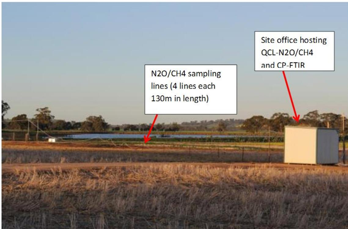
Figure 10 Close path N2O and CH4 sampling system
