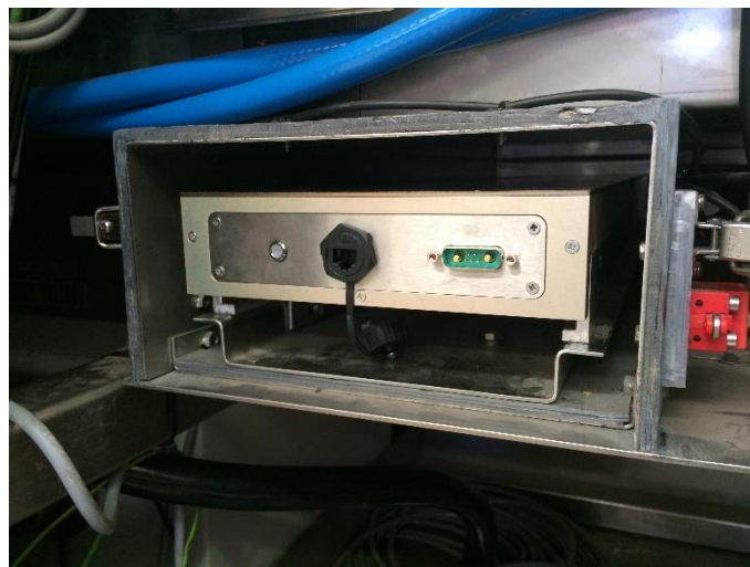
Figure 3: Dual energy detector installed in XR3000 inspection machine
