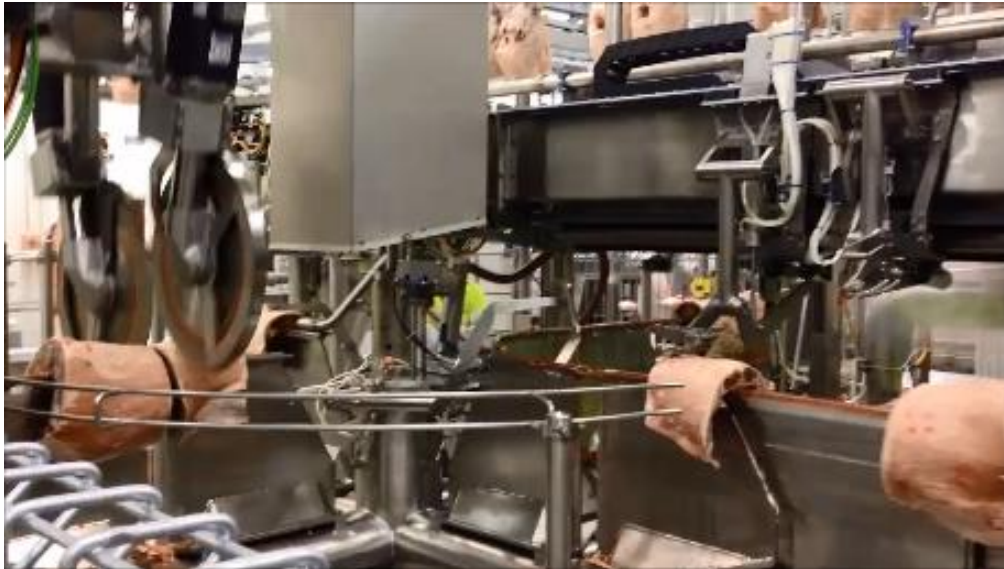
Figure 6: Separation of rack and loin in left of image prior to transfer to further processing of flap and chine removal in right hand side of image.
