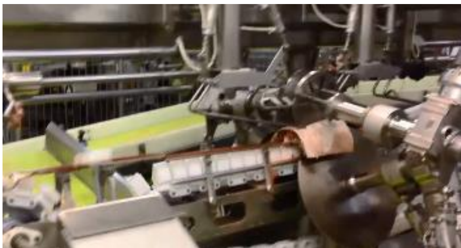
Figure 29: Fully automated chining unit installed as part of commercial LEAP IV middle system
