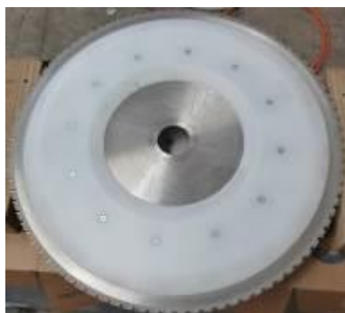
Figure 26 Modifications made to reduce the production and spread of saw dust
