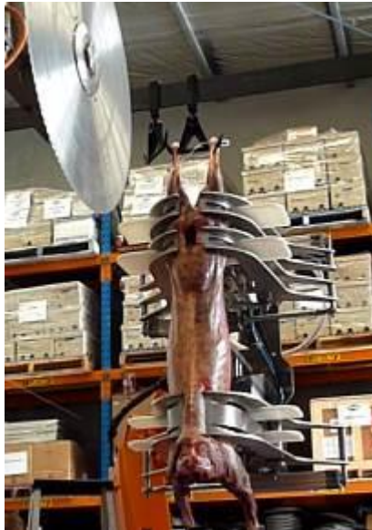
Figure 27 Trials with Blade running in an anti clock wise direction, with Gripper in 'long' configuration
