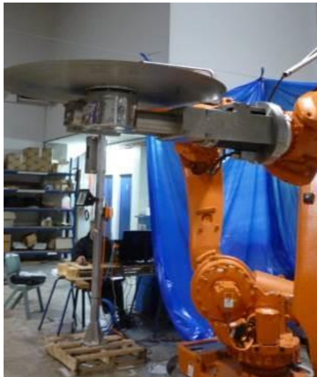
Figure 31 Horizontal cutting saw blade mounted to the original motor and robot
