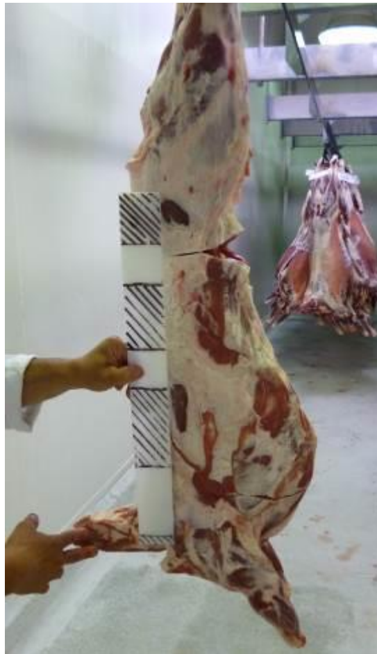
Figure 6 Gripper finger location compared to cut lines
