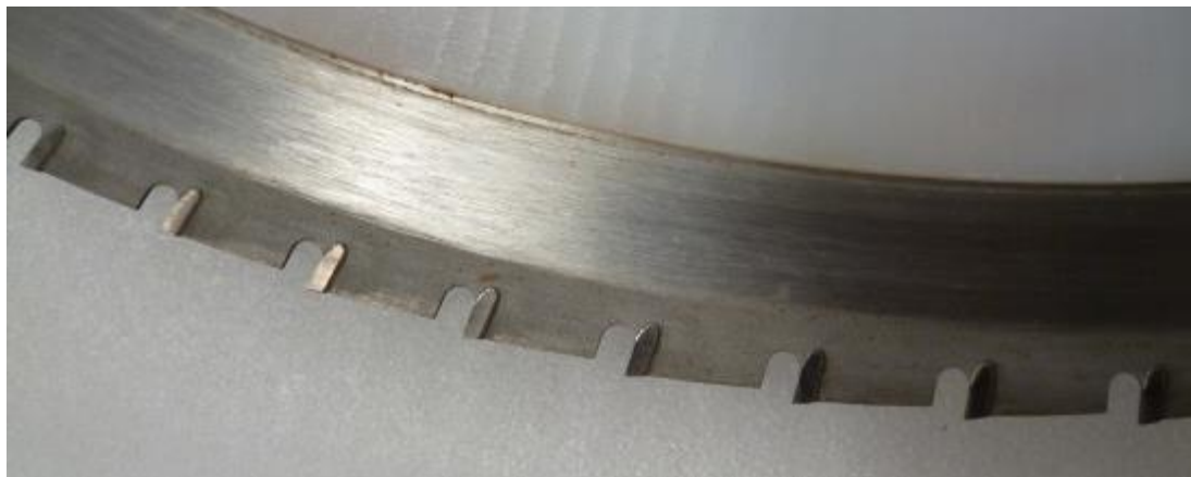
Figure 22 720mm Toothed Blade setup and profile
