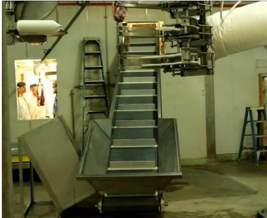
Figure 39 Leg exit rail, blade sterilisation tank and product exit conveyor
