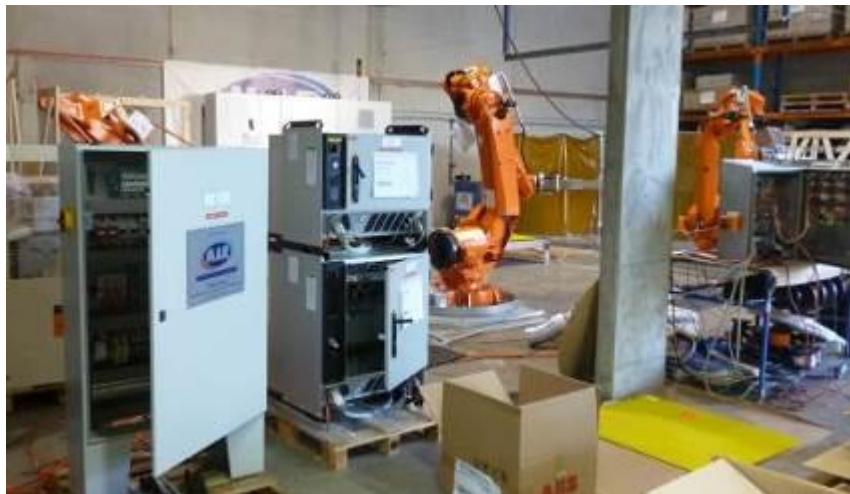
Figure 18 Control and operator panels interfaced to Robot Controllers
