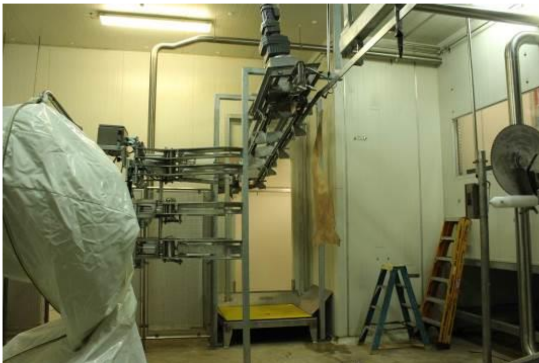
Figure 346 Carcass infeed conveyor with safety mat and carcass gripping robot in the foreground.
