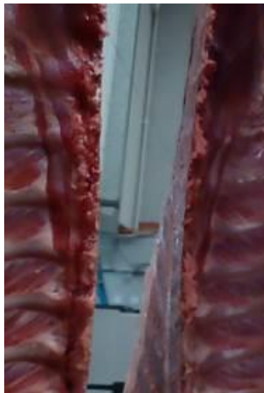
Figure 24 Bone and meat dust produced using toothed blade
