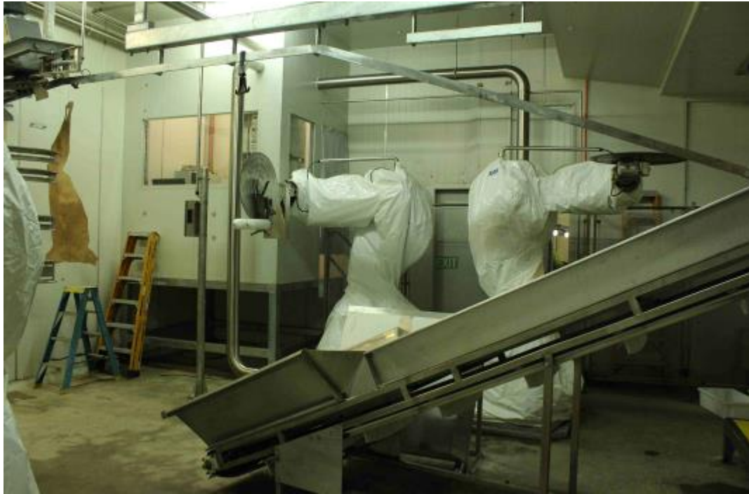
Figure 37 The two cutting robots with the carcass camera on the left and product exit conveyor on the right.
