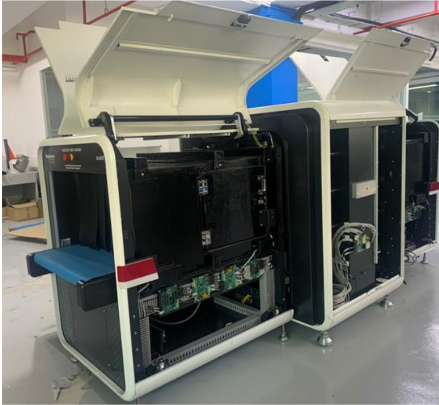
Figure 8: Photograph of the MEXA CT system with its covers open for servicing,
