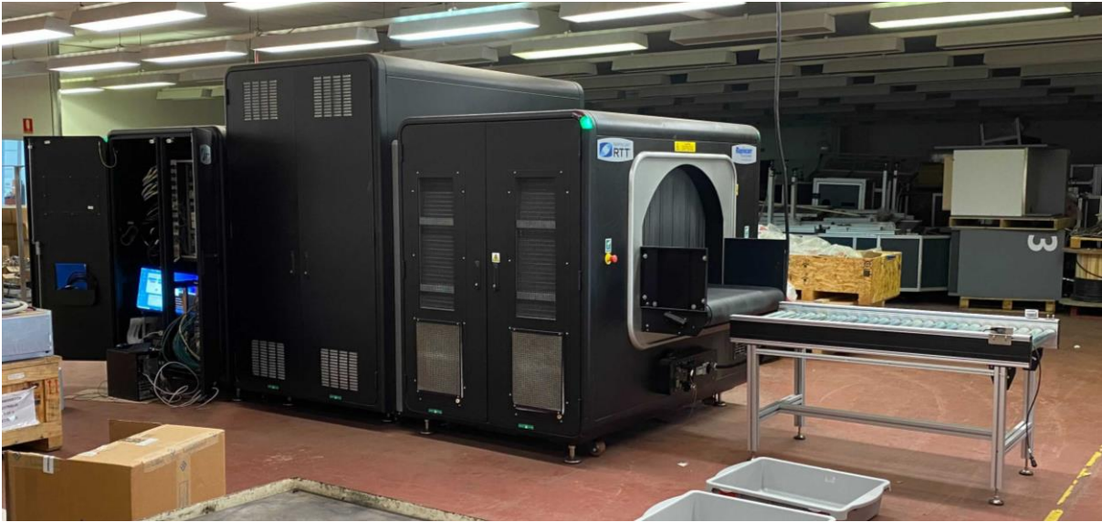
Figure 17: RTT110 installation for carcass scanning.
