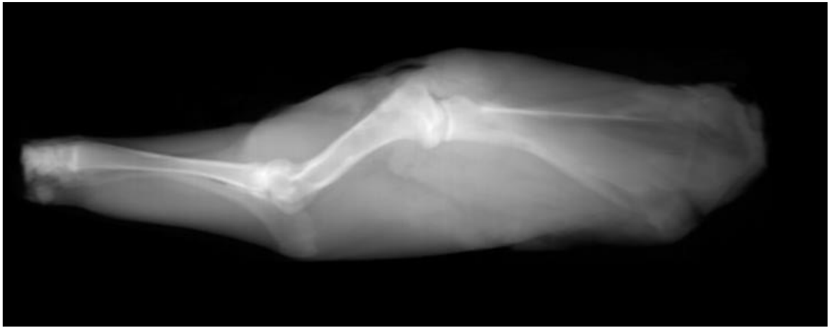
Figure 21: A 2D projected image from the 3D scan of a beef leg. The projection displays the bone, lean and fat distribution in different shades of grey.
