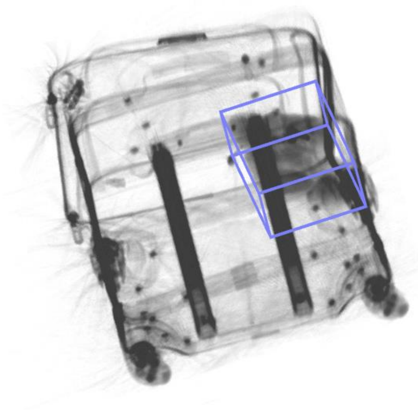
Figure 5: Detection algorithm display for meat found in a passenger bag.
