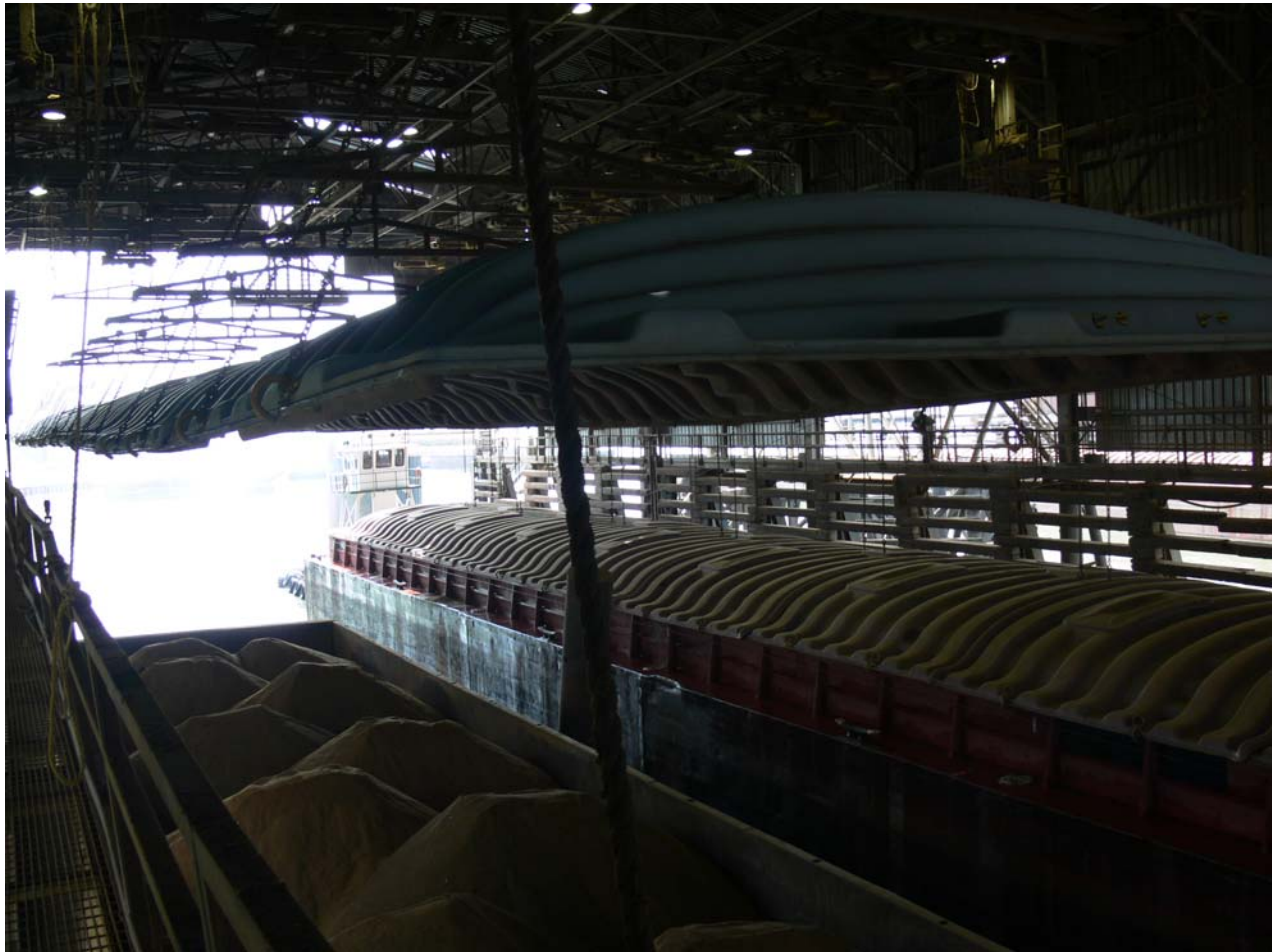
Plate 9 - Barge cover raised to permit unloading and thorough cleaning for identity preserved shipments of either grain or byproducts.
