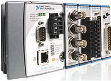
Figure 4.2: National Instruments CompactRIO PAC
