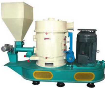
29. Zhengyuan Powder Super Rotor Mill LHW 2000 – used for food and fibre (similar to other turbo mills, but cheap)
