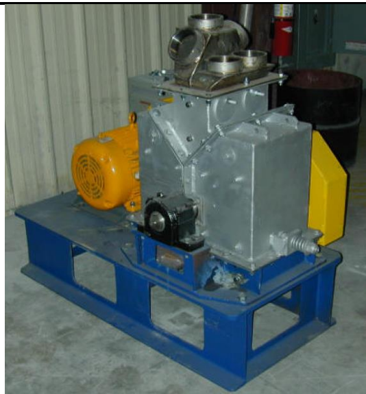
17. Dense Phase Jet Mill – mainly used for toners and very fine powder markets
