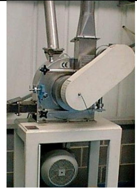
28. Neue Herbold ZM 800 Pulverizer – used for plastics has a static and a rotating disc
