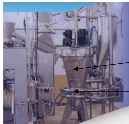
36. Poittemill Group High Yield Pulverizer used for food and minerals, essentially a crusher of Turbo-mill design.
