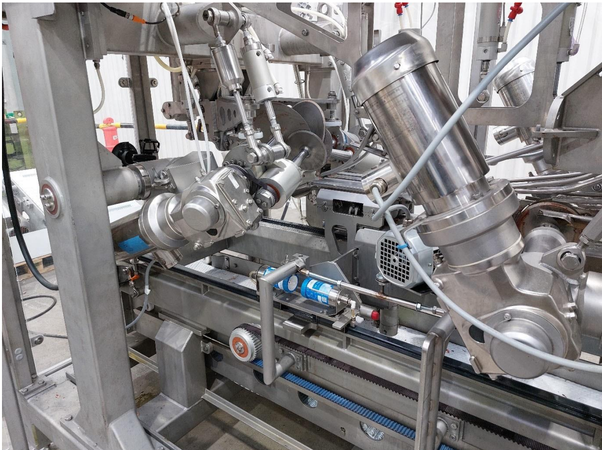
Figure 40: Eye of loin removal station - overall assembly
