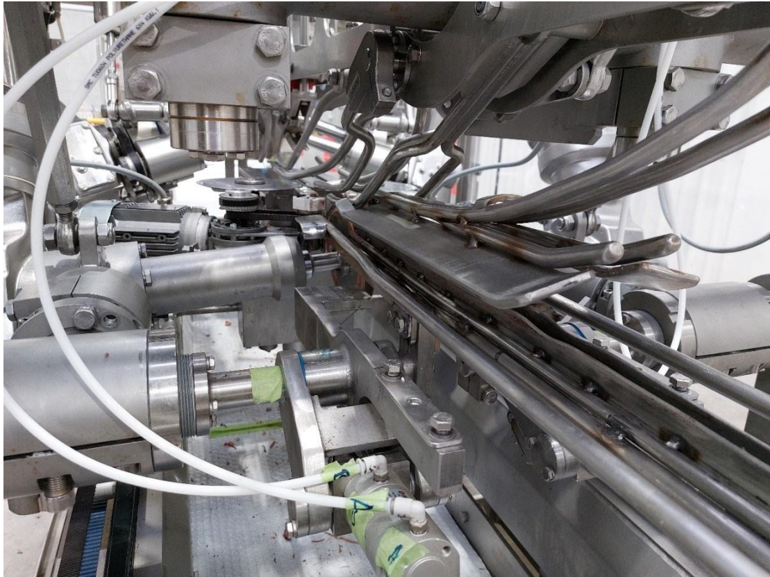
Figure 29: Loading zone. Showing scrapers and full length hold down.
