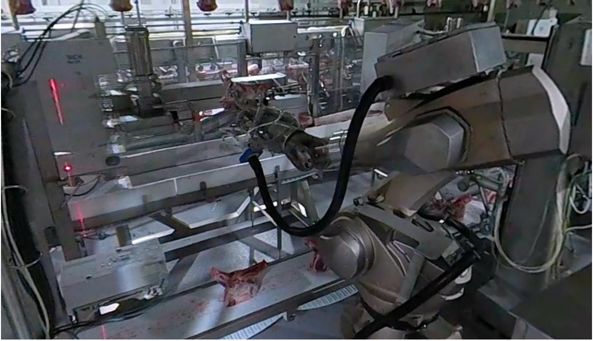
Figure 7: Forequarter processing robot and bandsaw
