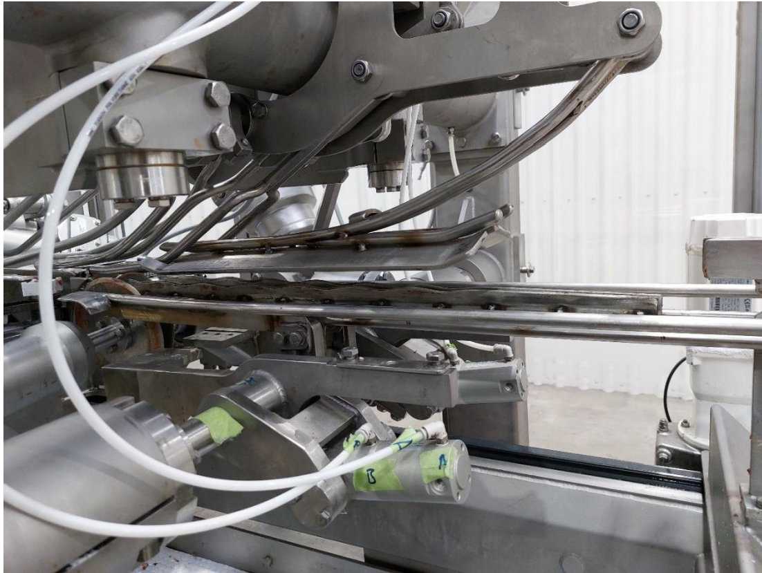
Figure 20: Loading zone, scraper, hold down. Shows the scallop scraper
