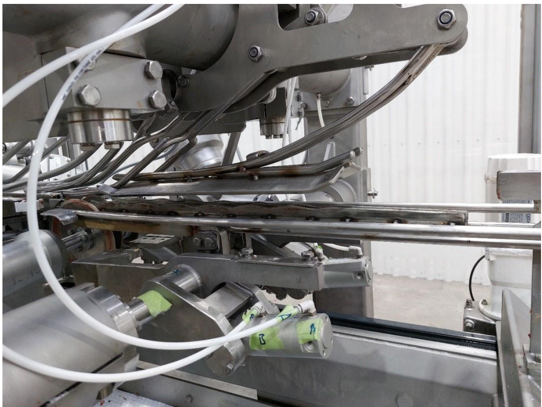
Figure 30: Loading zone, scraper, hold down. Shows the scallop scraper
