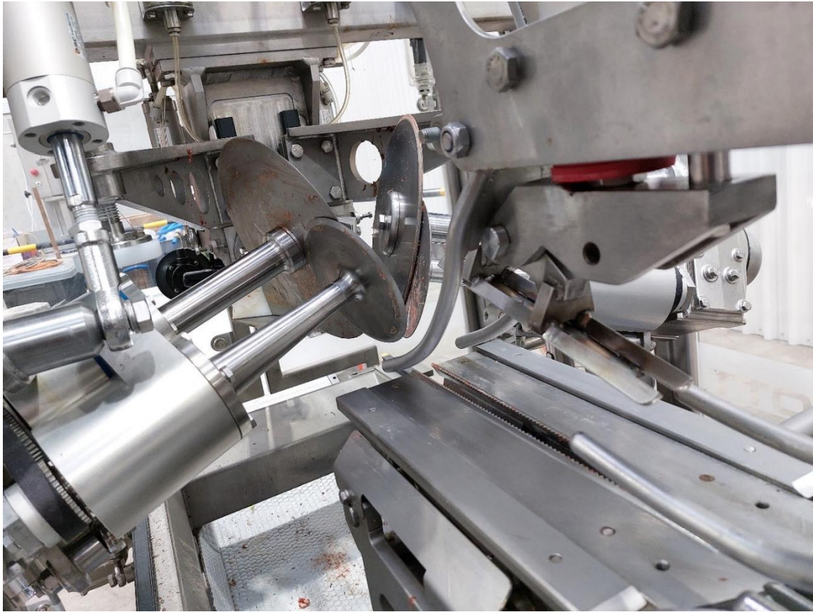
Figure 41: Eye of loin removal station showing blades detail including geometry between the blades that clears the button bones.
