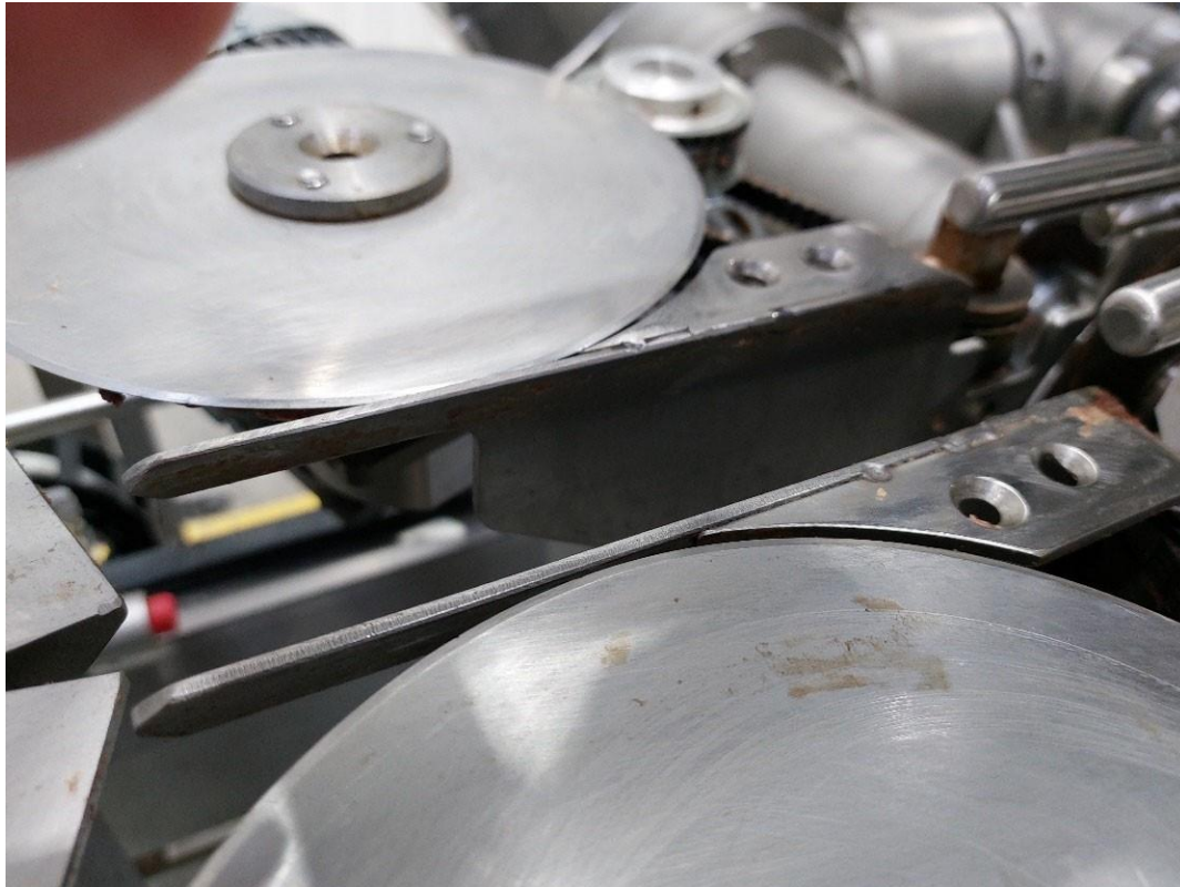
Figure 35: Tenderloin tail cutting blades and associated vertical height setting guides
