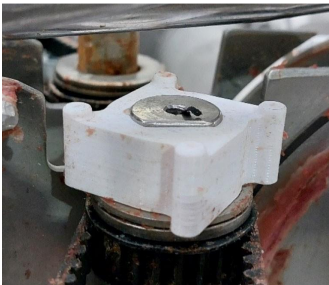
Figure 2: An example of one of the versions of TL removal wheel that was 3D printed
