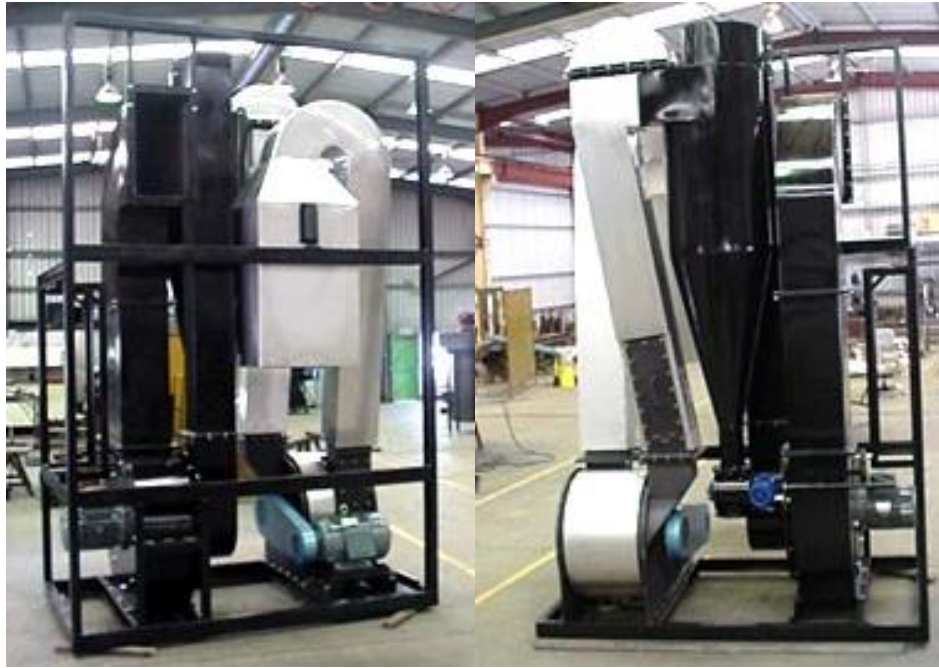
Figure 3.4: Images of an AKT packaged rendering system (KY1). Source: https://www.akt-kix.com
