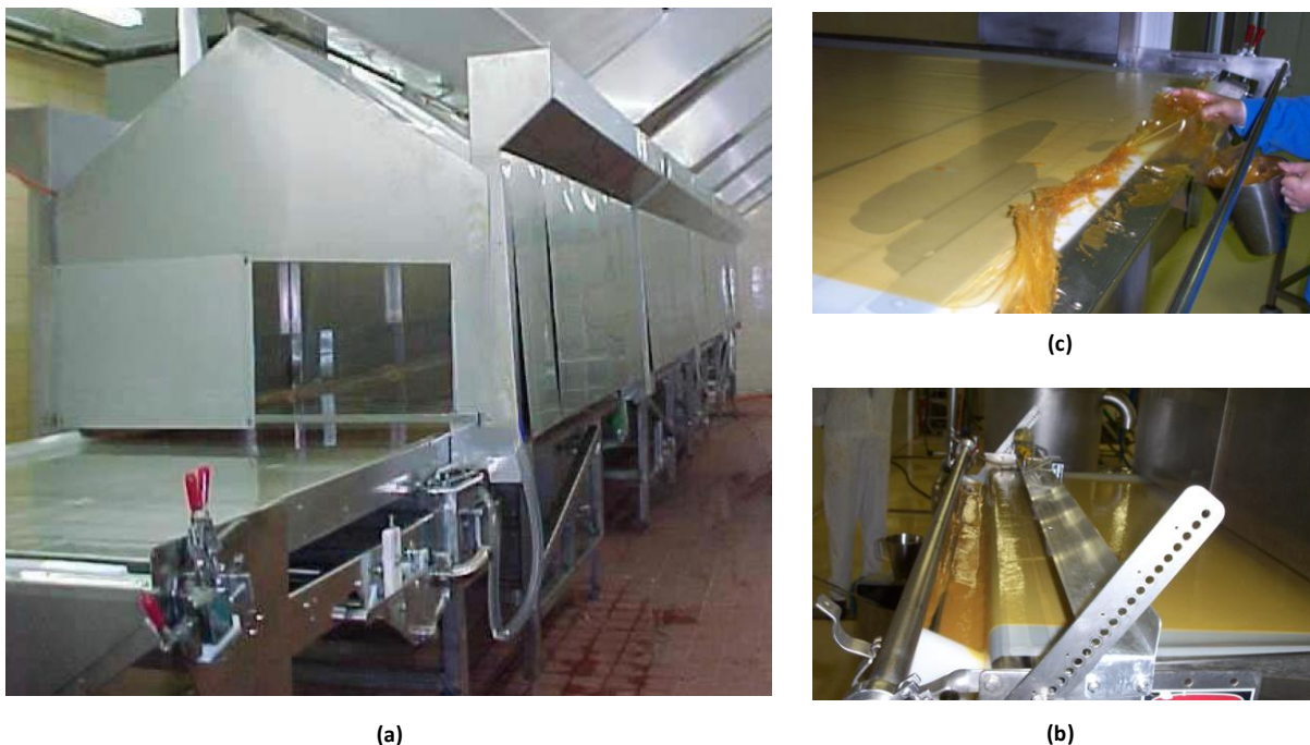
Fig. 10. Photos of (a) commercial scale RW dryer facility (RWD5 Model, MCD Technologies, USA), (b) wet-feed entry end of the dryer, and (c) dried-product exit end of the dryer (Sabarez and Chessari, 2006).
