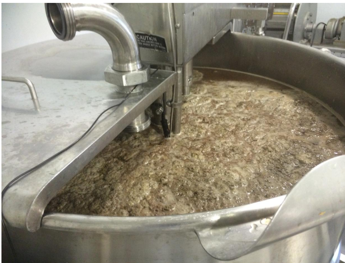
Fig. 2. Cooking of beef liver samples with hot water in a 300 L heating vessel.
