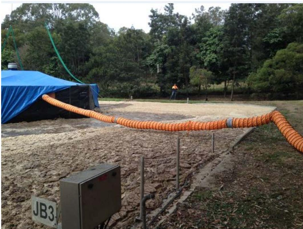
**Photo 5:** Pilot test rig setup over the aerobic ponds ready for odour collection.
