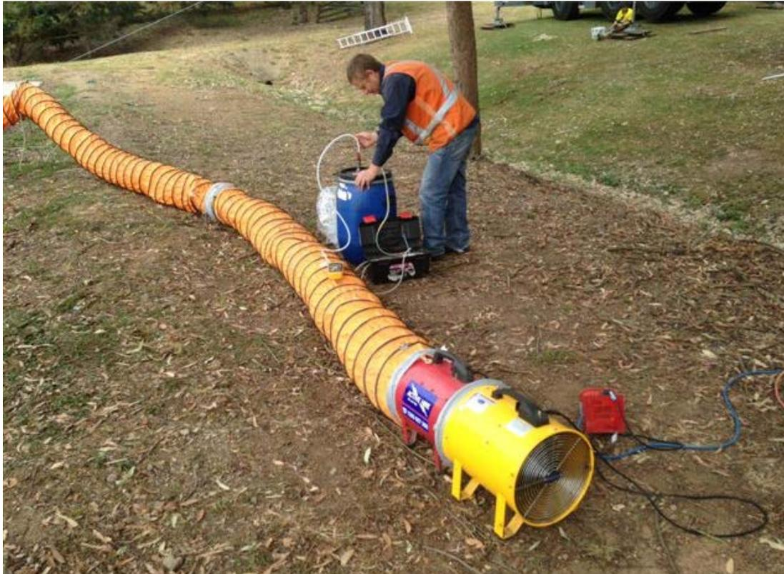
**Photo 4:** Setting up exhaust extraction fans for collection of odours.
