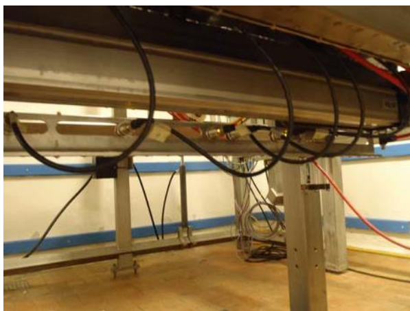
Fig 9: Spinal column cavity location lug proximity sensors(used to energise location lugs as guide traverses spinal column cavity- refer Fig 10)
