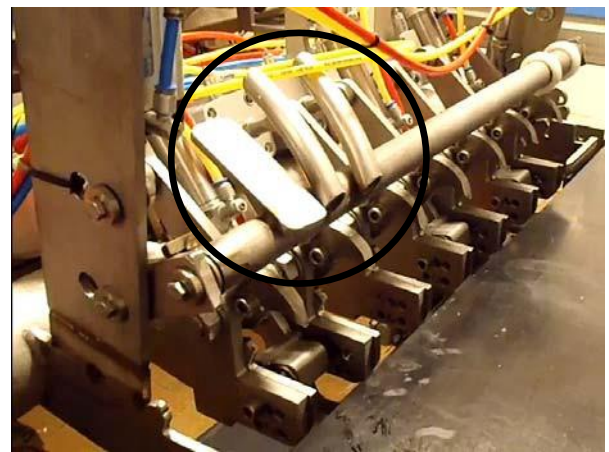
Fig 12: Guides to accommodate differences in width between the varying shapes of the round rib and flat ribs
