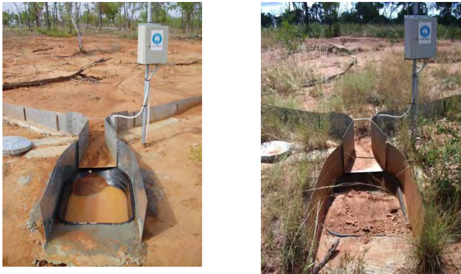
Figure 25: Visual evidence of the high suspended (left) and bedload (right) measurements observed at Flume 3
