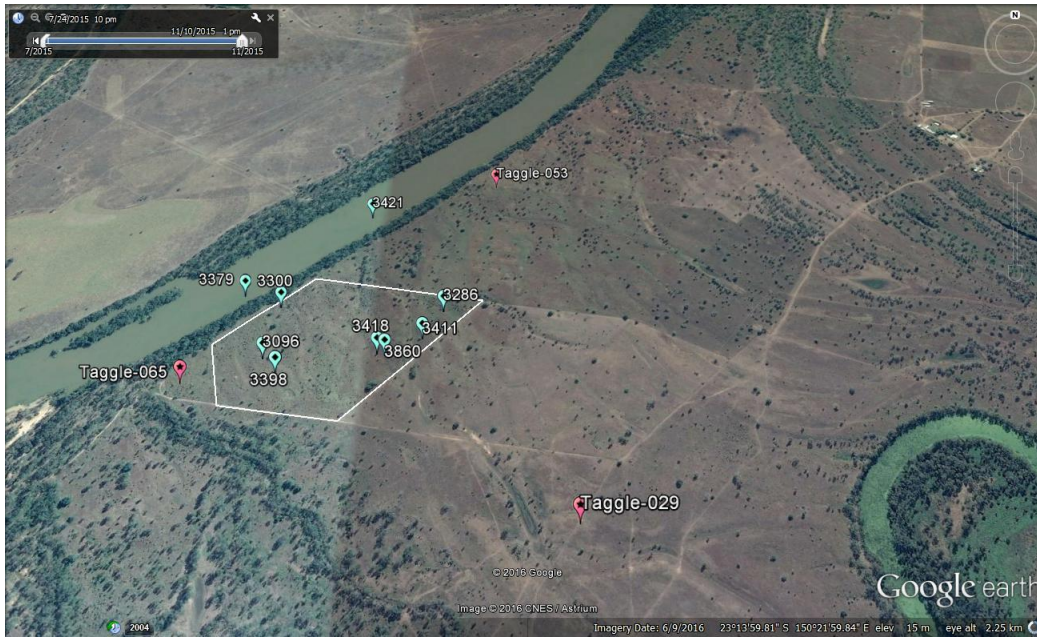
Figure 10 - Google earth image (16m above sea level) of the calving paddock with the white line showing the perimeter and the green teardrops showing the derived locations for the 9 Calf Alert devices. Also shown, as pink teardrops, are three of the four Taggle receiver towers.
