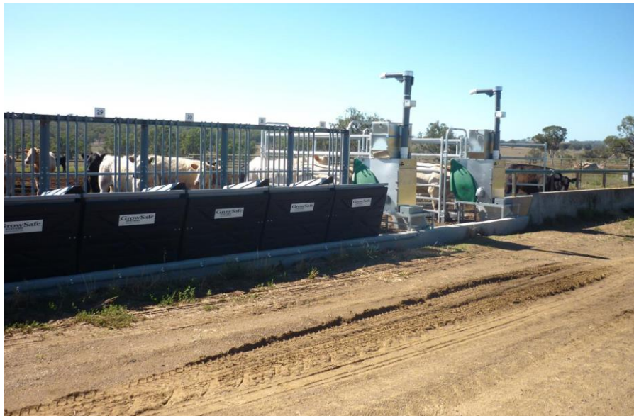
Figure D6. GreenFeed emission monitoring units fixed in the feedlot pen where cattle access their main ration from the GrowSafe feed bunks beside; as used of screening industry cattle for feed efficiency and emissions
