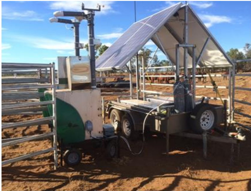
Figure D15. Greenfeed unit operation (solar powered) at Dungowan, Augathella May 2015.
