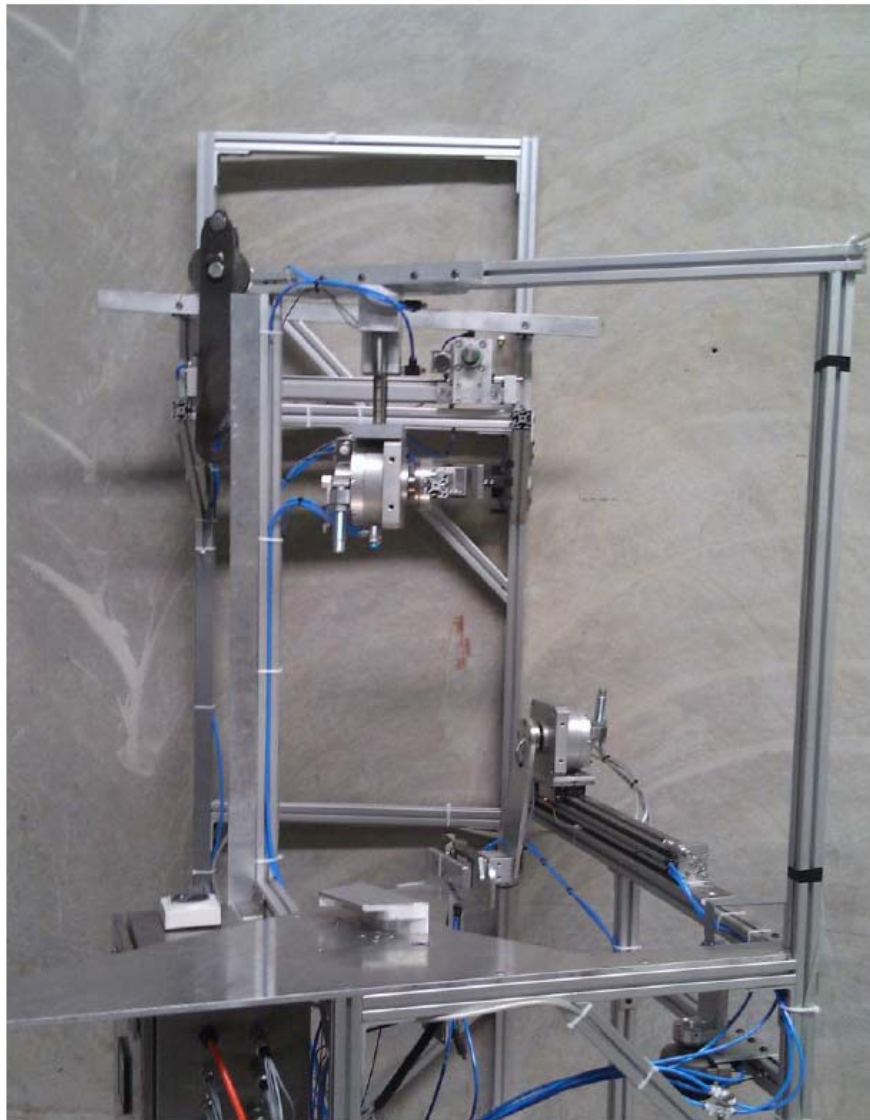
Figure 8: Automatic Shackle Loading System
