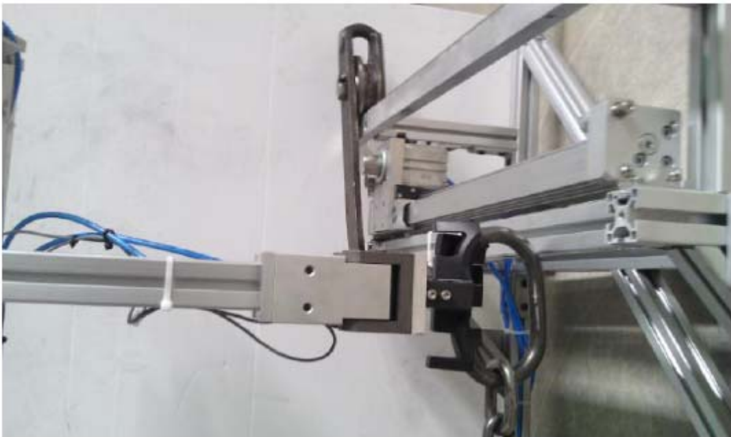
Figure 12: Shackle removal from bleed roller
