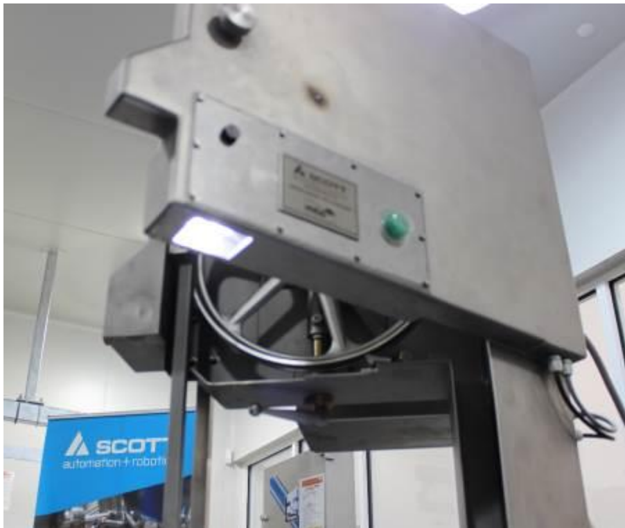
Fig.3 Custom double skin bandsaw door for housing the LED lighting system
