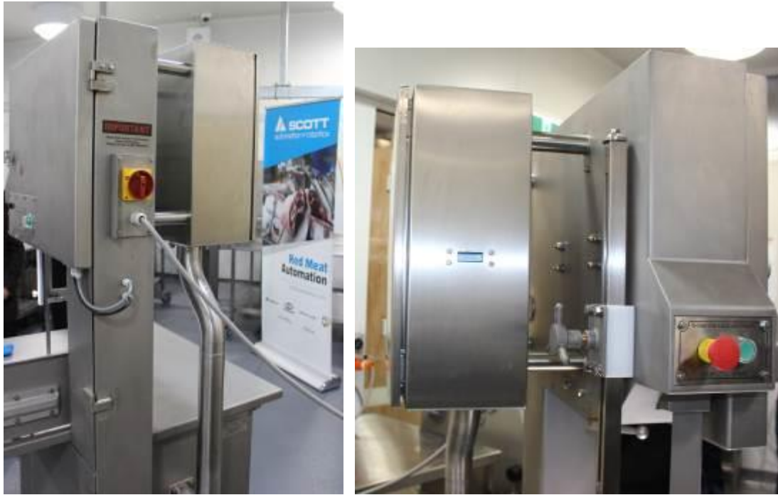
Fig.2 Electronics box fitted to the rear of the saw
