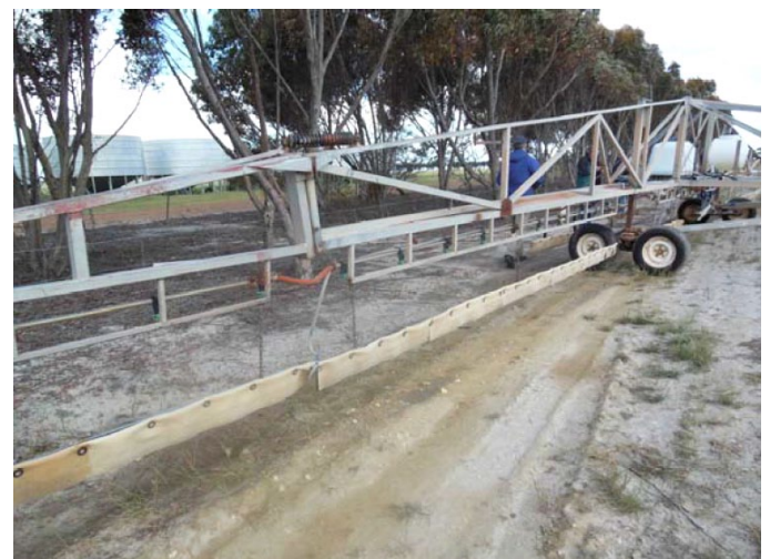
Figure 18. A blanket wiper may be a useful strategy for controlling weeds in biserrula by exploiting height differences between the biserrula and target weed.
