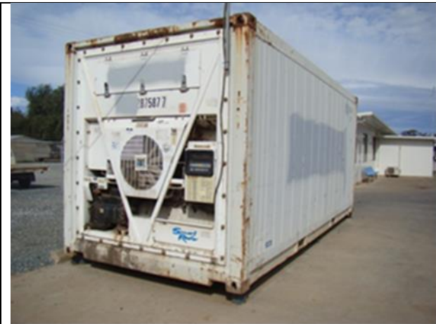
Figure 2 - Refrigerated shipping container
