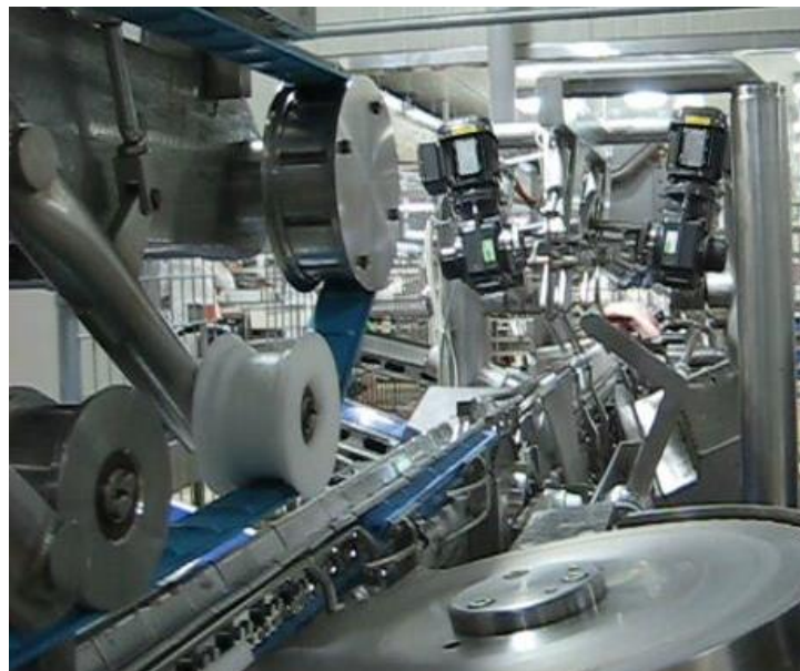
Figure 4: Chine station integrated into middle machine looking downstream from the flap cut station.
