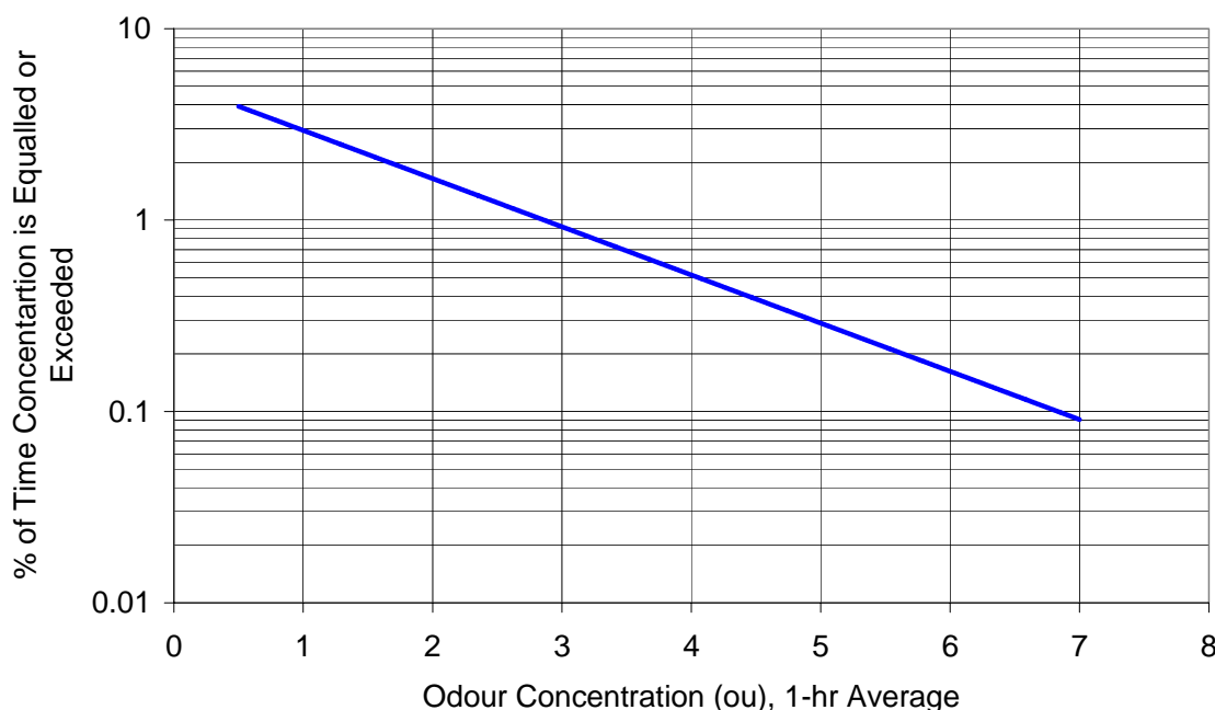
Figure 4.1: Hypothetical 'acceptable limit' curve of odour concentration vs frequency-of-exceedance (see text for discussion). Note: the actual concentration values in the graph are not proposed as actual criteria, but are for illustrative purposes only.
