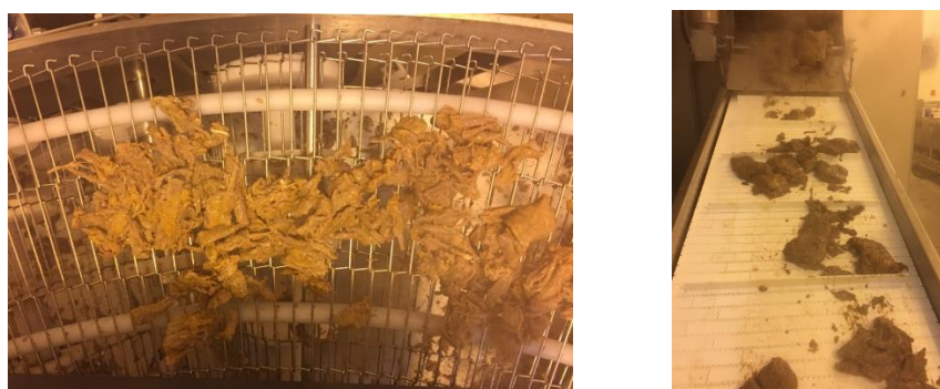
Figure 4: Photo of old and new conveyor belt to reduce yield loss
