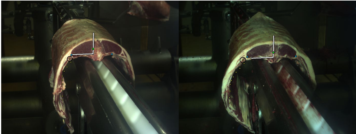
Figure 13. Currently the position of the front face of the product at camera 3 (half camera) is calculated from x-ray data and provided to the middle analysis. If this is incorrect (and it is incorrect by up to \pm 20\text{mm} ) then the image appears like the left-hand image where the projected axes do not align with the featherbone and the bottom of the product (see the right-hand side for where the axes should be). This error means that the pixel to mm calculation is off and so even if the eye meat is found correctly then the cut position will still be incorrect.
