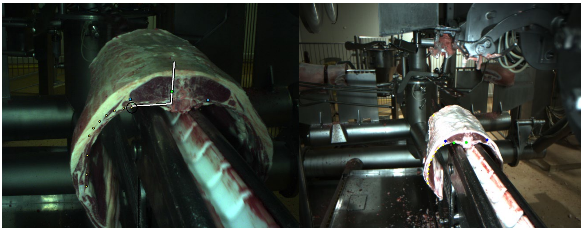
Figure 16: The left-hand side image shows the existing analysis using the provided product position, which shows the face of the loin being further forwards than expected. The right-hand side image is from the and has directly measured the product position.
