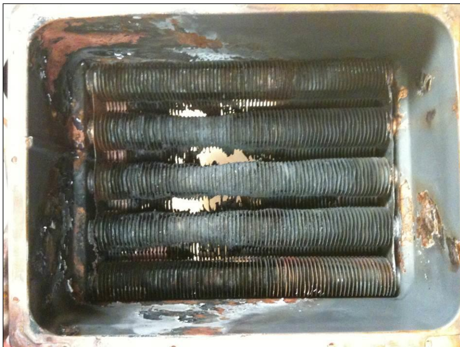
Figure 18: Gas HWS heat exchanger after failure.
