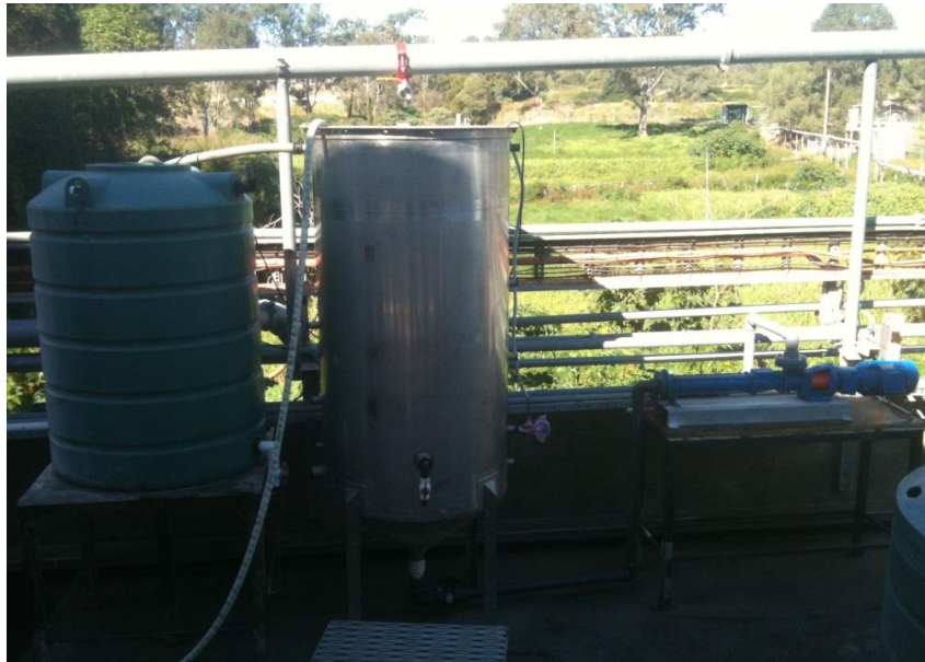
Figure 6: Wastewater feed collection system at TPAD demonstration plant host site in 2010.
