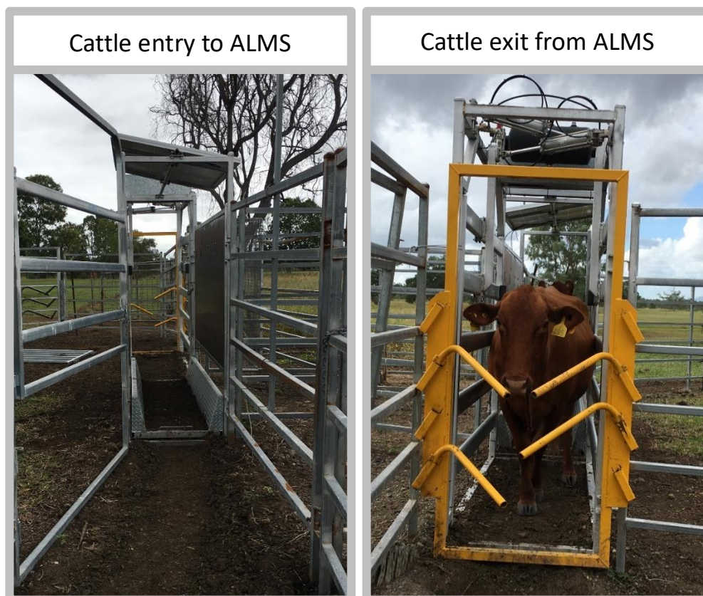
Fig. 9. ALMS entrance and exit, showing the spear gates at the ALMS exit to prevent animals returning back past the reader and weigh scales
