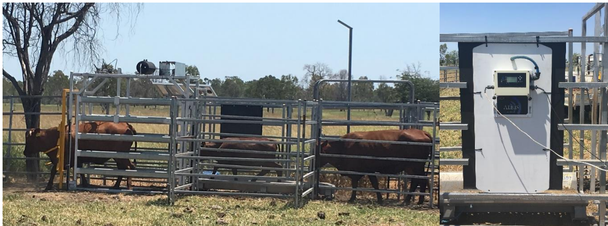
Fig. 11. Left: Initial auto-drafting unit attached to the walk-over-weigh platform used by the trial cattle. Right: RFID panel reader mounted on plywood to avoid the read-range extending the entire length of the metal panels
