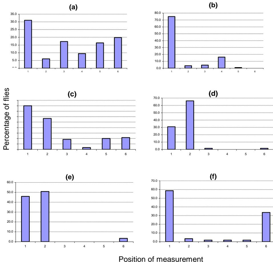
**Figure 13.** Distribution of flies under different light regimes. a) Light below netting, b) Light under table (no direct light), c) White light on side 1; d) White light from side 1 with silhouette on side 1; e) Infra red on side 1, f) Moonlight on side 1. Positions on the x axis are: 1 = top of the cage; 2 -5 = sides; and 6 = bottom.
