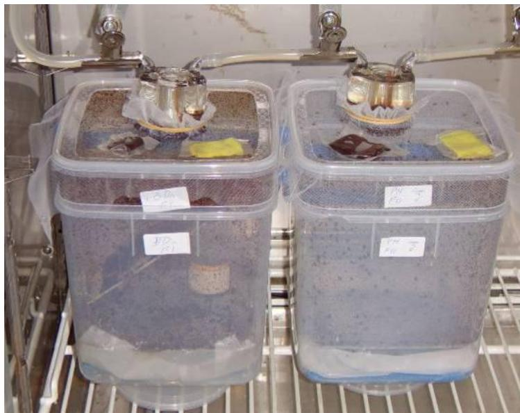
**Figure 4.** An iteration of rearing system incorporating membrane feeders providing ad lib blood at the top of the cage with blood heated to 37°C by water recirculated from a water bath. Dung pats for egg laying (and feeding if required) is provided in a Petri dish in the bottom plastic container with mesh of top cage pushed down on top. Bottom cage also contains saturated Wettex® sponge to maintain humidity and keep faeces and eggs moist
