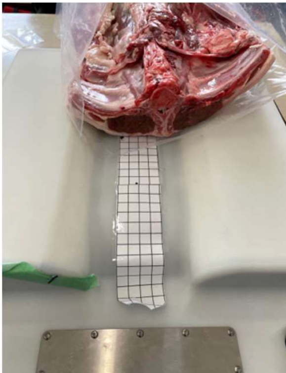
Figure 2. photo showing optimal positioning of a saddle on the sensor. Notably the spine is positioned into the groove of the sensor enclosure.
