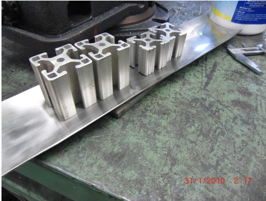
Fig 16: Static Compression Test - various Limit Blocks.
