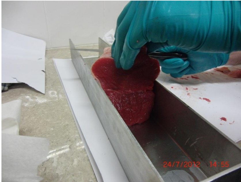
Fig 14: Static Compression Test - Meat Loading into Trough.
