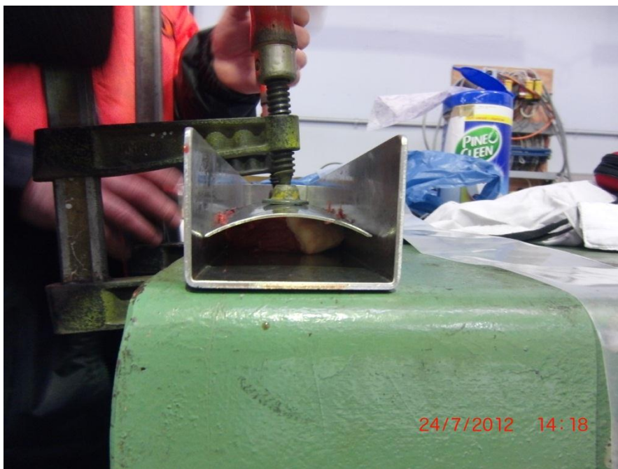
Fig 15: Static Compression Test - Meat Clamped.
