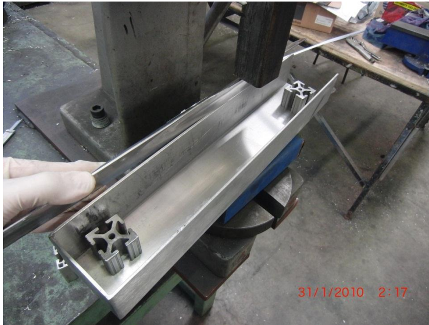
Fig 13: Static Compression Test - Meat Trough and Limit Blocks.
