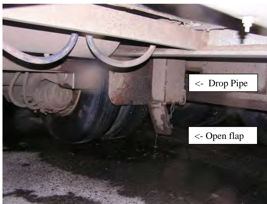
Figure 38 – Some drop pipes from livestock vehicles can be closed thus preventing loss of effluent while travelling through urban areas.
