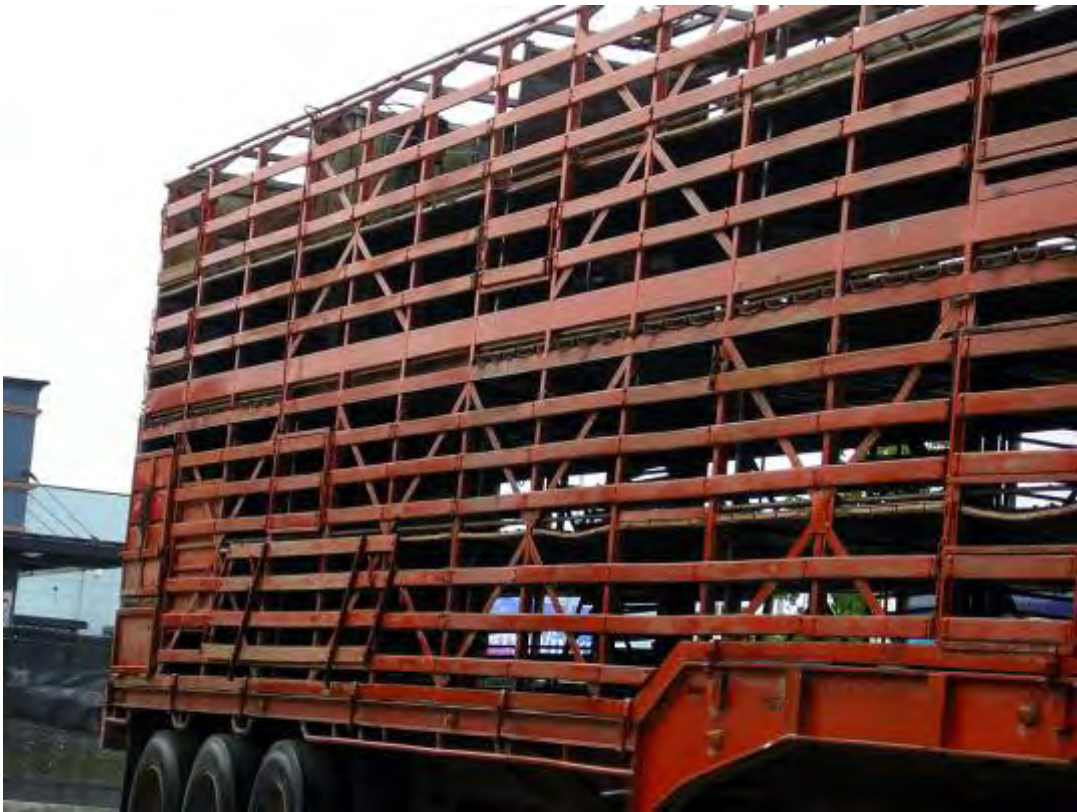
Photograph 23 – Old Sheep Trailer with Large Gaps
