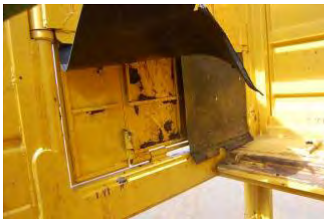
Photograph 20 – Rubber mats prevent effluent spillage through gates
