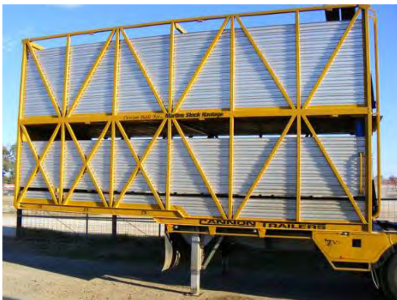
Photograph 12 - Trailer with solid panels and ventilation gaps
