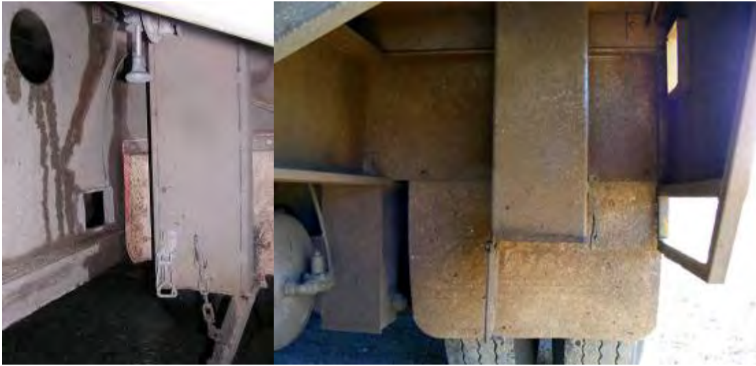
Photograph 18 – Temporary effluent containment system (shut-off valve)
