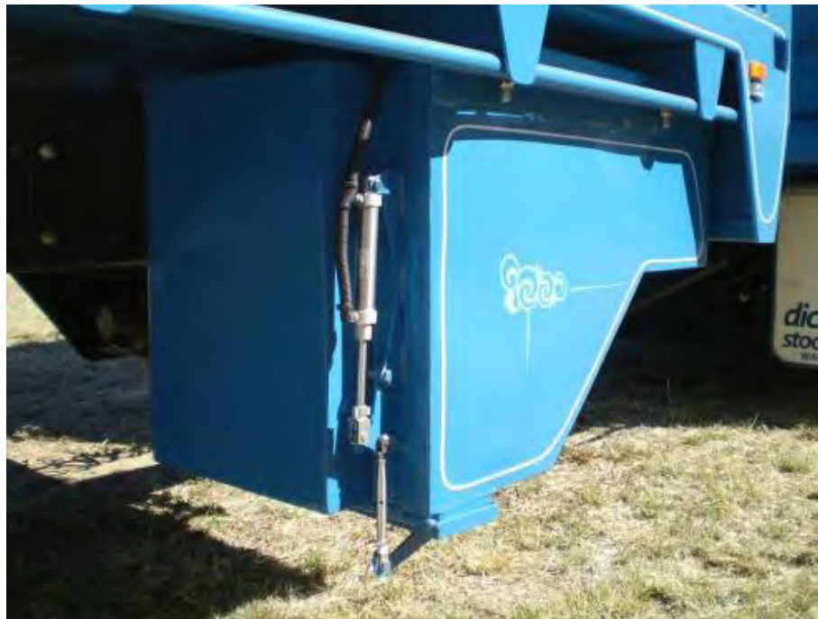
Photograph 22 – Effluent holding tank with cabin-actuated opening valve
