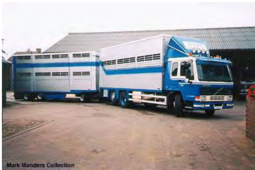
Photograph 3 – European cattle trailer – Includes ventilation system and water system
