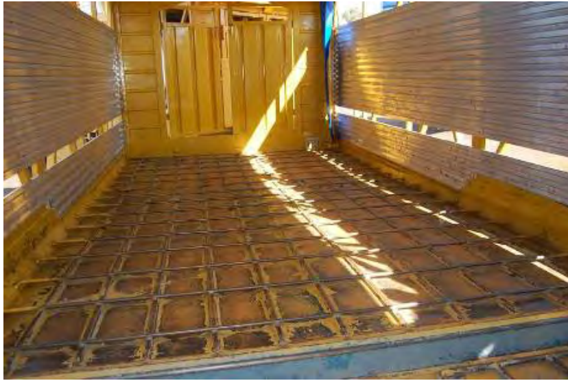
Photograph 13 – Trailer floor is sloped to allow effluent to drain to the back
