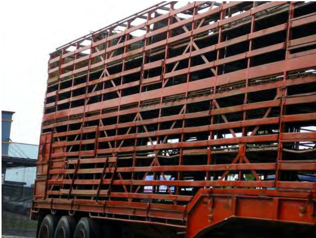
Figure 36 – Limb protrusion is possible through wide gaps in side panelling in old-style sheep transport trailers
