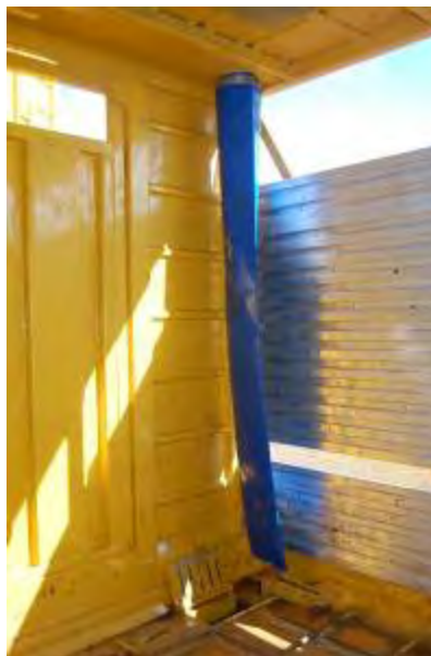
Photograph 16 – Effluent drainage from the top deck to the bottom deck via conduit
