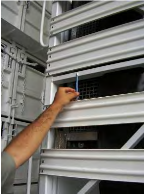
Photograph 29 – Gaps in New Combination Sheep / Cattle Trailer Rails (approx 120 mm)
