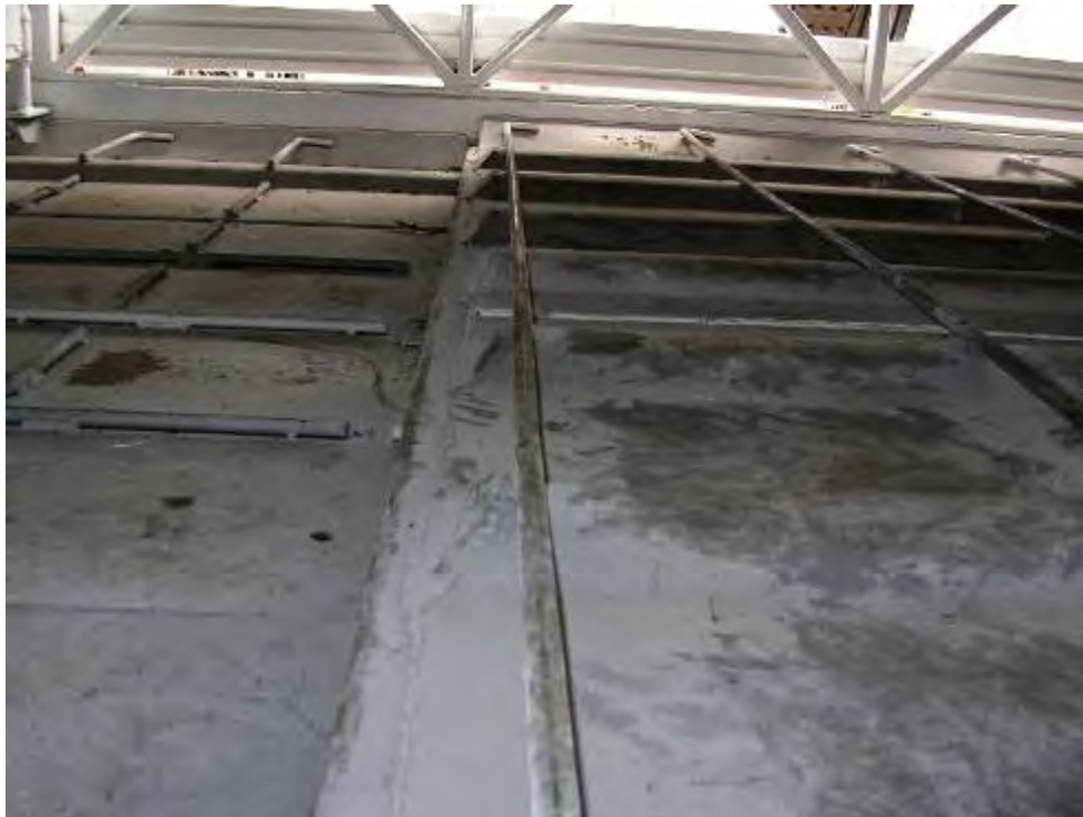
Photograph 31 – Solid floor in new combination sheep /cattle trailer
