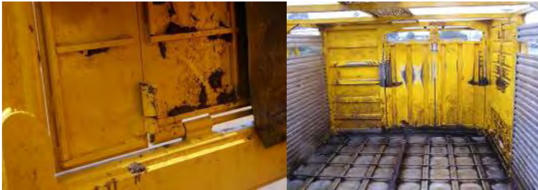
Photograph 19 – Unsealed gates on livestock trailers
