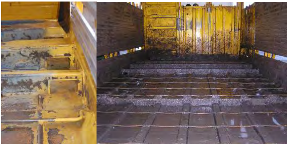
Photograph 14 – Effluent drains along sides of trailer
