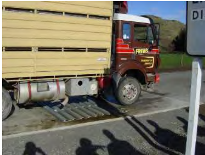
Figure 40 – Stock truck dumping effluent over grate (New Zealand)
