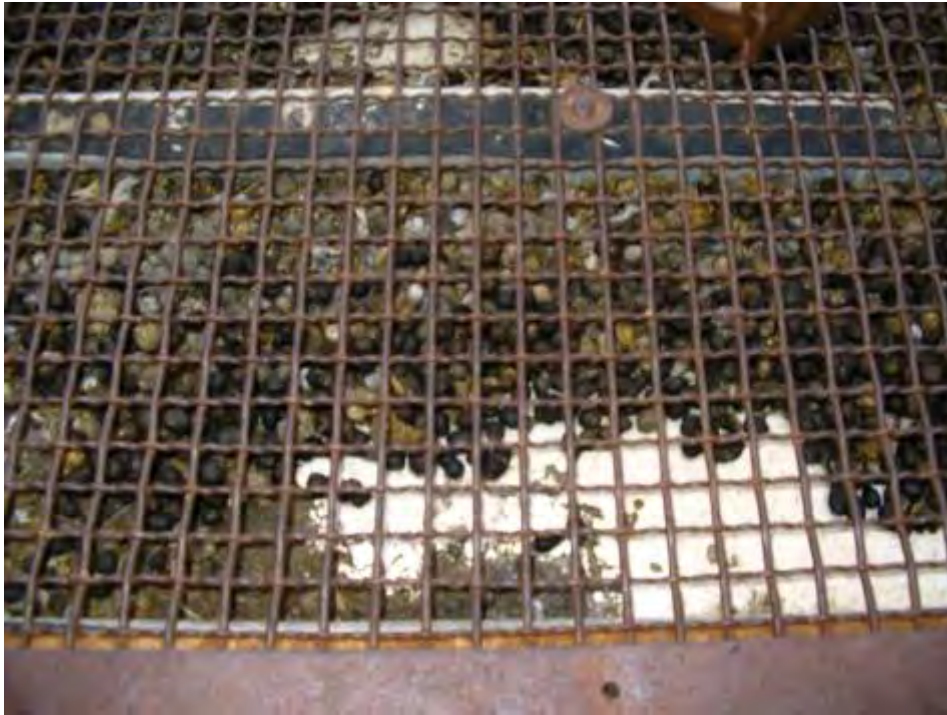
Photograph 30 – Upper deck of older-style sheep trailer showing manure containment
