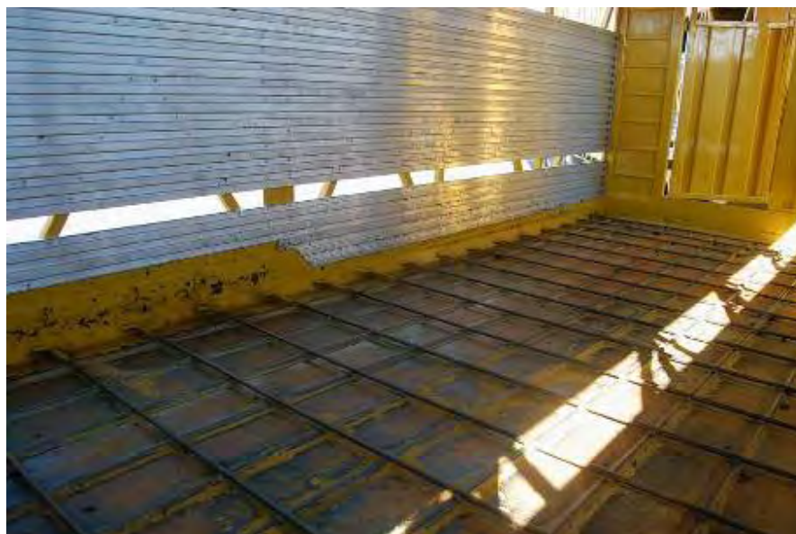
Figure 37 – The sidewalls and floors of many new livestock transport are now designed to allow a reasonable accumulation of effluent in the base of the livestock trailer.
