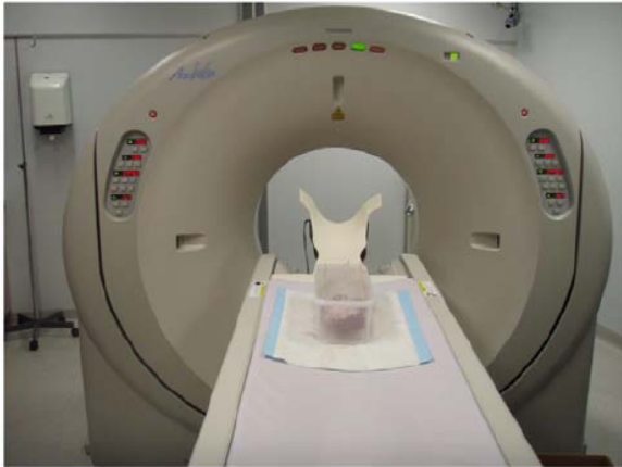
Figure 3: Toshiba Aquilion 16 slice CT system with cold cube roll ready for measurement
